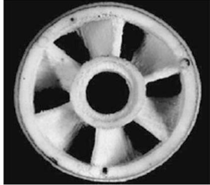
**Fig. 7.6** Sintered zirconia vertical walls [18]
