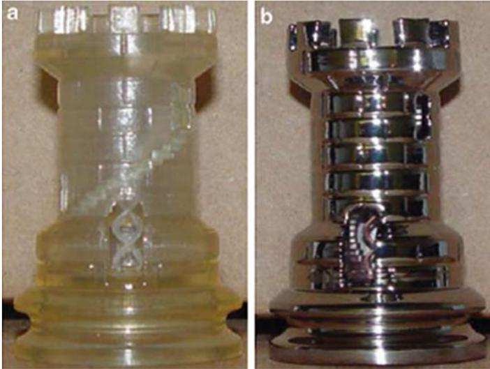
**Fig. 14.10** Stereolithography part (a) before and (b) after chrome plating (Courtesy of Aircraft Plating)
