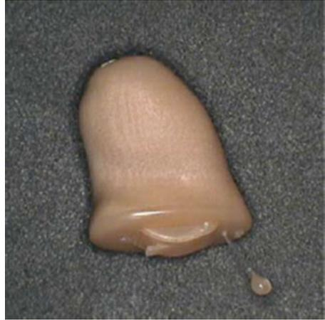
Traditionally, an impression is taken of a patient's ear, which is then used as a pattern to make a mold for the hearing aid shell. An acrylic material is then injected into the mold to form the shell. Electronics, controls, and a cover plate are added to complete the hearing aid. To ensure proper operation and comfort, hearing aids must fit snugly, but not too tightly, into the ear and must remain in place when the patient talks and chews (which change the geometry of the ear).
