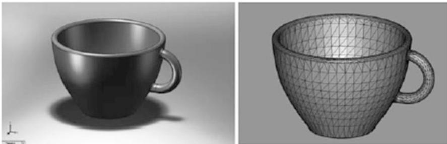
**Fig. 2.2** A CAD model on the *left* converted into STL format on the *right*
