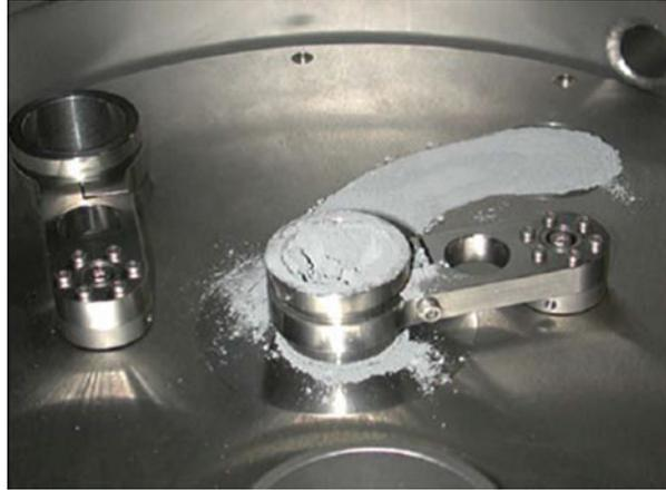
ceramic powders, in addition to melting of metal powders. Another unique characteristic of the 3D Systems machine is its use of a roller to spread and then compact powder, making it the only manufacturer which can directly change the powder bed packing density on-the-fly.
