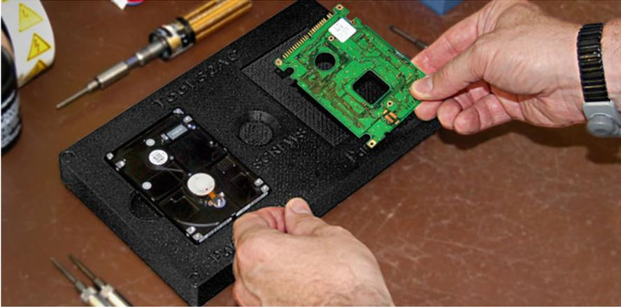
**Fig. 18.9** A hard drive assembly jig (Courtesy of Javelin javelin-tech.com)
