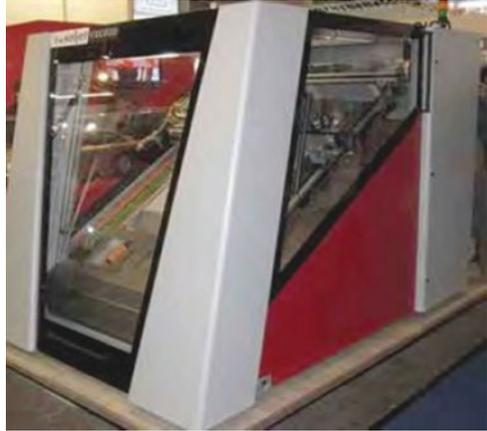
described earlier. A photo of the VXC800 is shown in Fig. 8.4. For this machine, the layer thickness is 150–400  $\mu\text{m}$  and they use 600 dpi print heads. The surface area of the inclined plane is  $500 \times 850 \text{ mm}$ .
