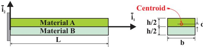
**Fig. 13.22.** Cantilevered bi-material beam under uniform temperature field.
