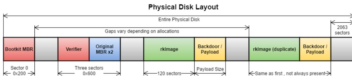
*Figure 5: Physical Disk Layout written by DEBUGFILE.sys*
