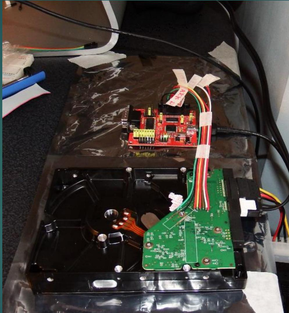
I'm using a TIAO USB multi-protocol adapter for JTAG / SPI
