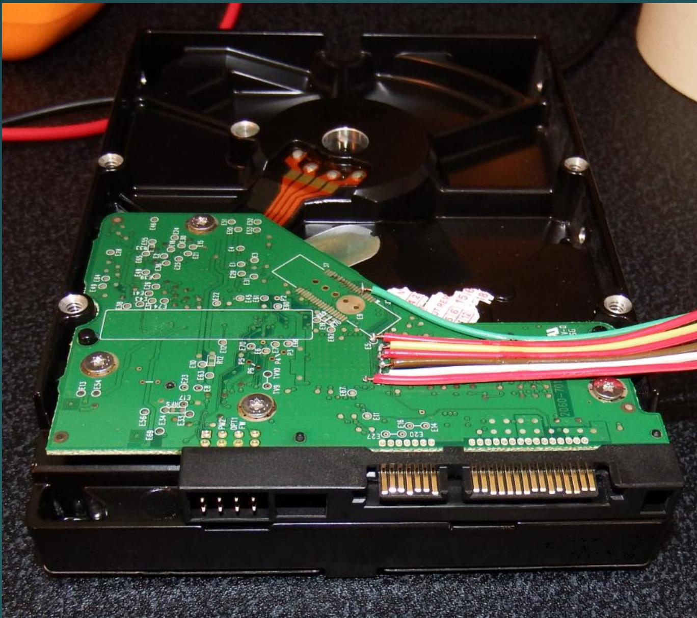
JTAG and SPI wires are soldered directly to the PCB
