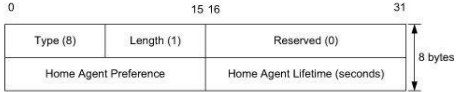
Figure 8-47. The Home Agent Information option indicates the preference and amount of time in which the sender of the option is willing to be considered a home agent for Mobile IPv6. Larger values of the Home Agent Preference field indicate a more desirable home agent. The Home Agent Lifetime field gives the number of seconds during which the sender is willing to be an HA.
