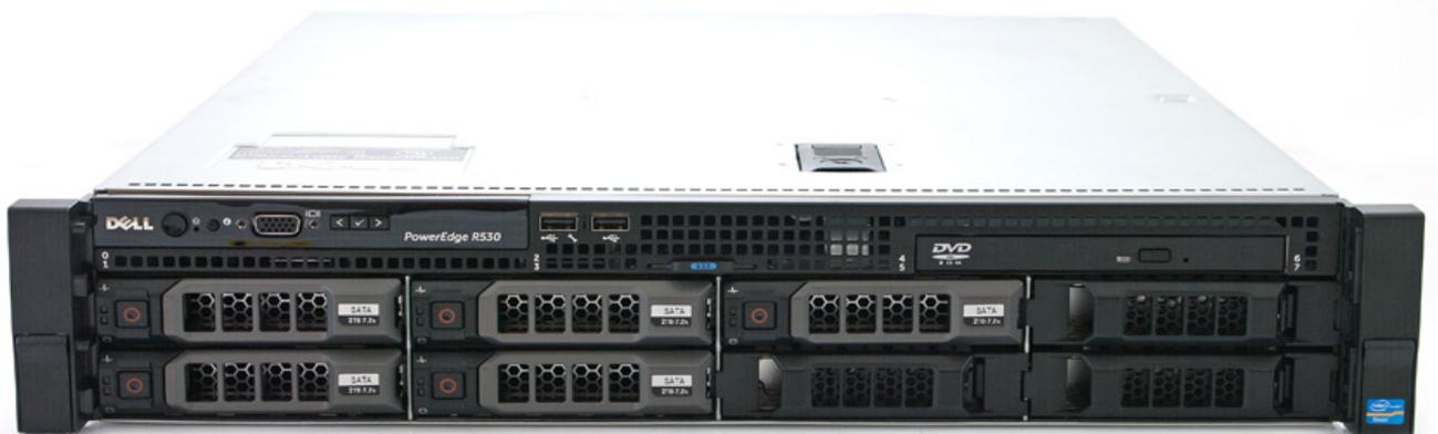
Figura 3-2: Frontal del servidor *Dell Poweredge R530* (extraído de [46])
