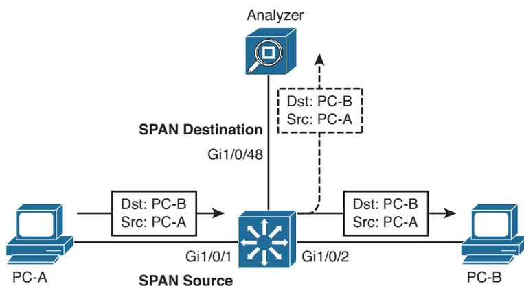
**Figure 16-1** Using Local SPAN to Monitor Received Traffic
