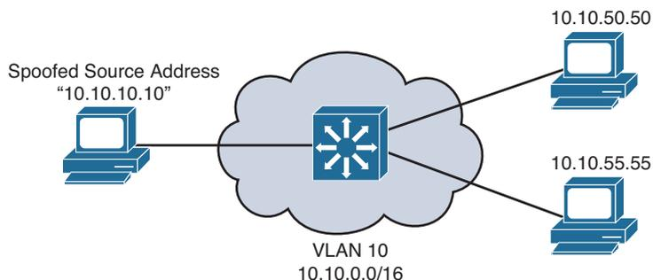
**Figure 21-1** Using a Spoofed Address Within a Subnet
