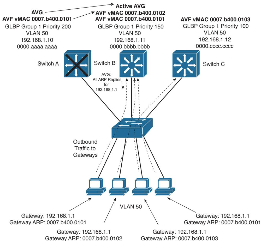
**Figure 18-4** How GLBP Reacts to a Component Failure
