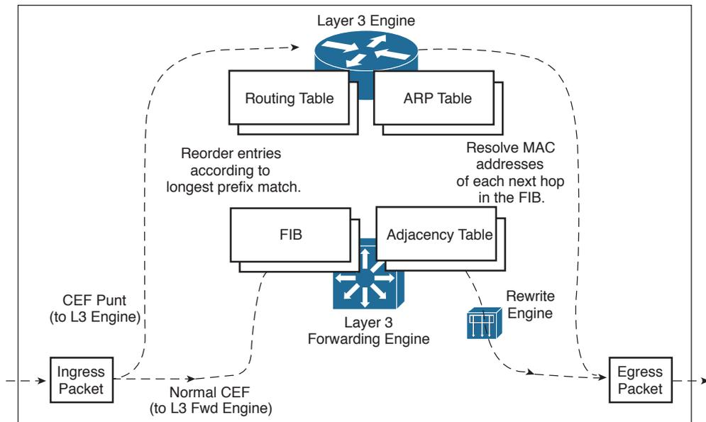
**Figure 11-3** Packet Flow Through a CEF-Based Multilayer Switch
