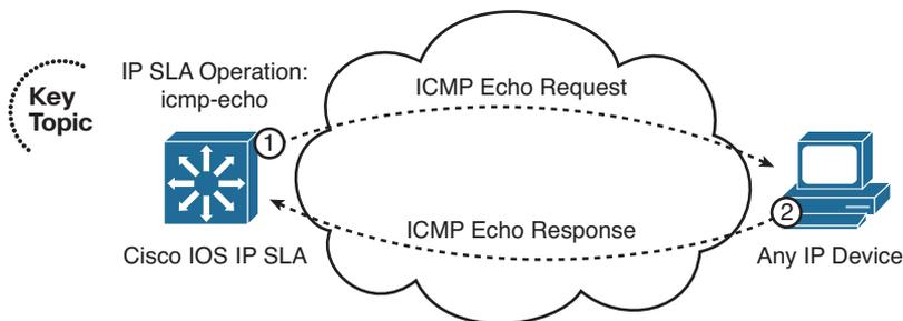
**Figure 15-1** IP SLA ICMP Echo Test Operation
