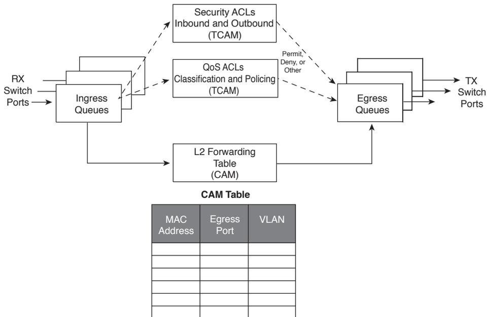
**Figure 2-3** Operations Within a Layer 2 Catalyst Switch
