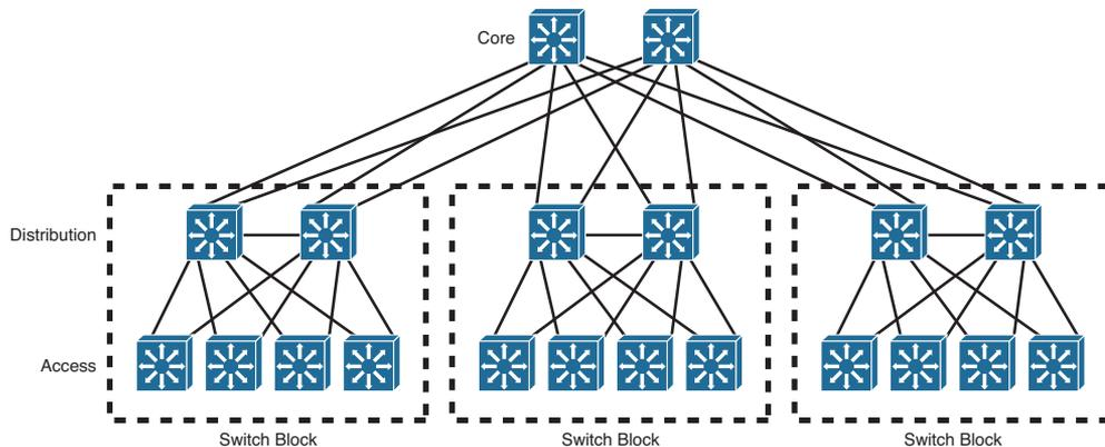
**Figure 1-12** *Network Growth by Adding New Switch Blocks*
