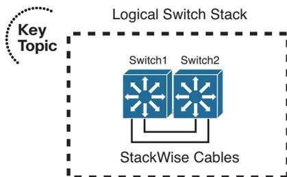
**Figure 17-6** *Creating a Logical Switch with StackWise*
