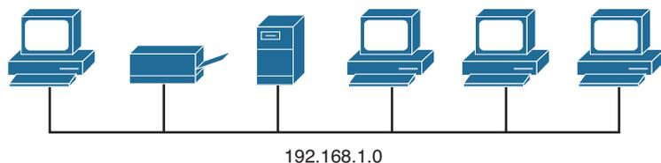
**Figure 1-1** *Simple Shared Ethernet Network*
