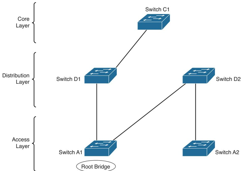
**Figure 7-3** *Final Spanning-Tree Structure for the Campus Network*
