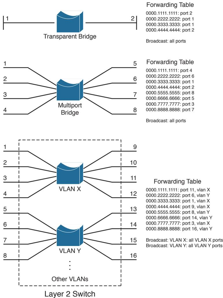
**Figure 2-1** A Comparison of Transparent Bridges and Switches
