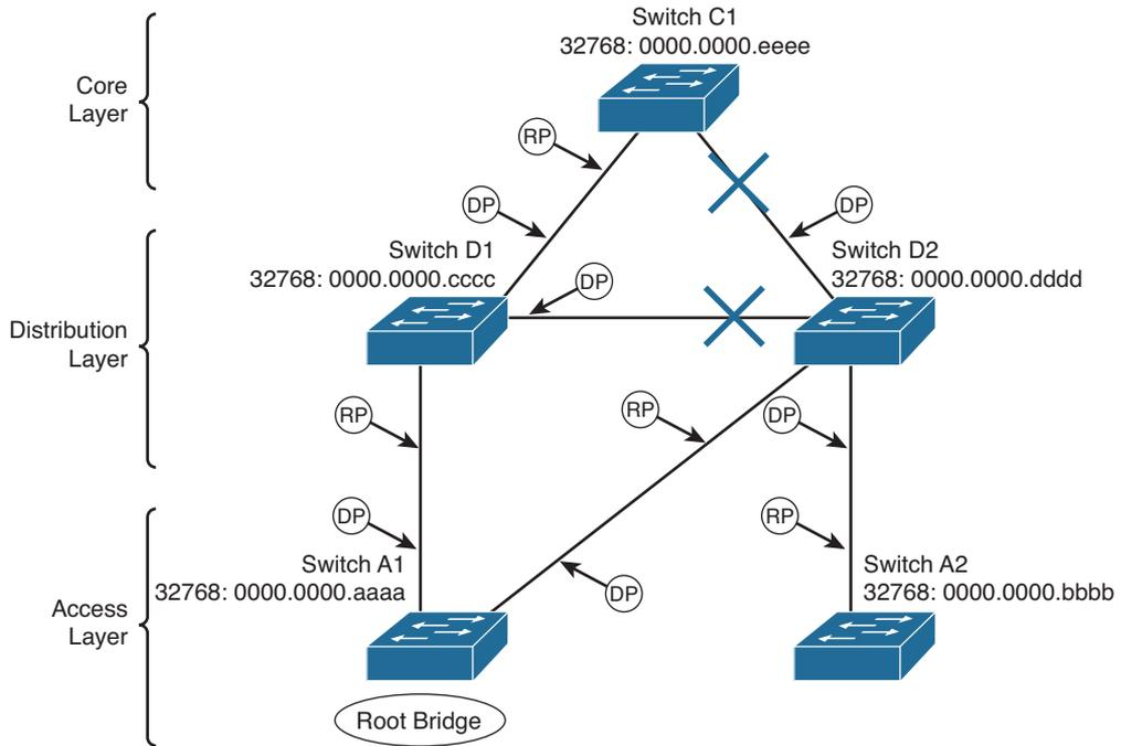
**Figure 7-2** Campus Network with STP Converged
