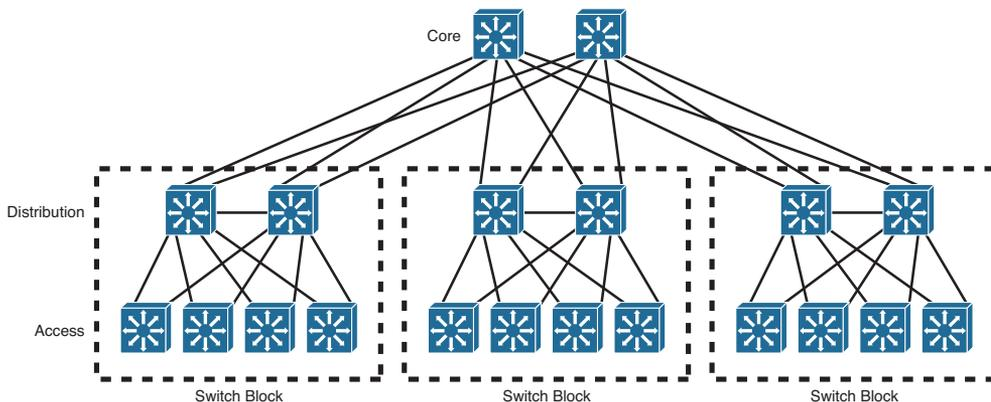
**Figure 17-4** *Traditional Redundant Switched Network Architecture*
