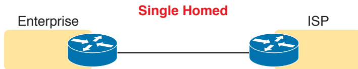
Figure 12-4 Single-Homed Design: Single Link, One Home (ISP)
