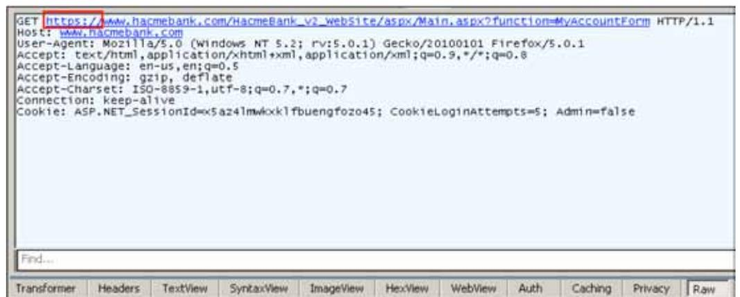
Figure 8. Figure shows the browser automatically modifies the request so that the connection attempt is made over HTTPS.
