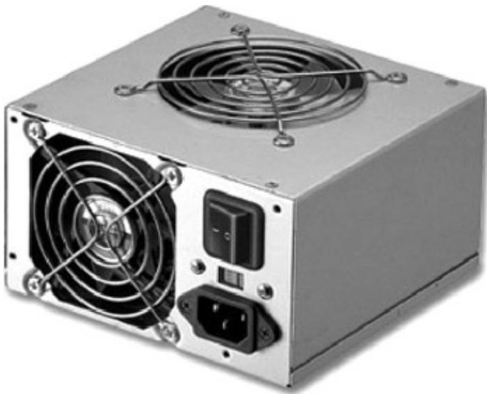
Figure 5-5: ATX power supply
