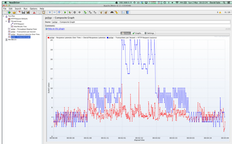
FIGURE 8-10: This combined graph view shows response times versus requests per second.
