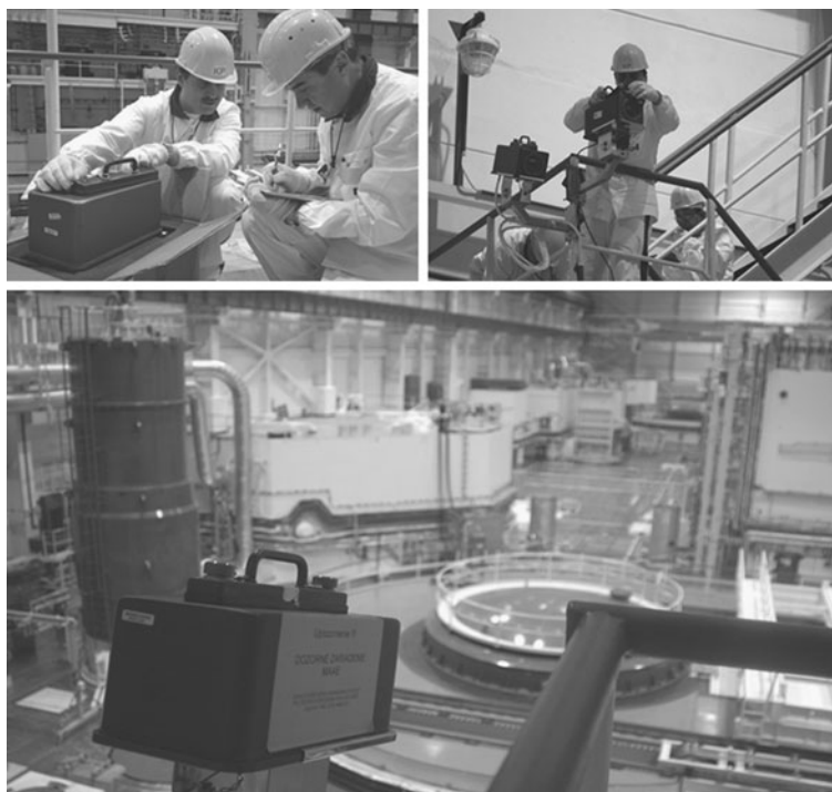
Fig. 1 Inspectors setting-up surveillance cameras in a nuclear plant ( first row ). A camera's view ( second row ) (© D. Calma/IAEA)
