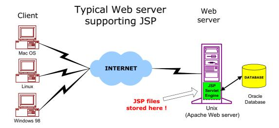
JSP source code runs on the web server in the JSP Servlet Engine. The JSP Servlet engine dynamically generates the HTML and sends the HTML output to the client's web browser.
