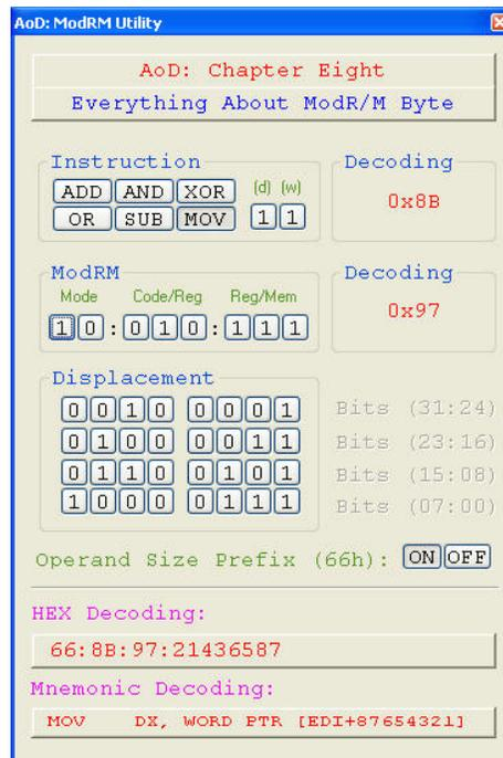
Figure 10.8: Example Two : Decoding The ModRM Byte
