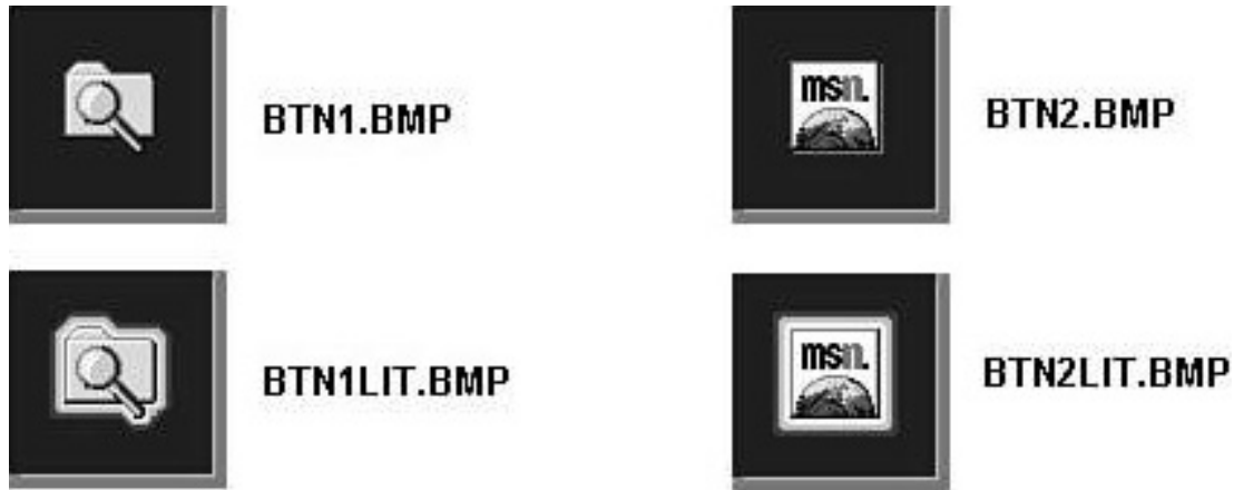
Figure 4.19 The BITMAP1 program uses these four bitmap resources to simulate light-up bitmap areas.
