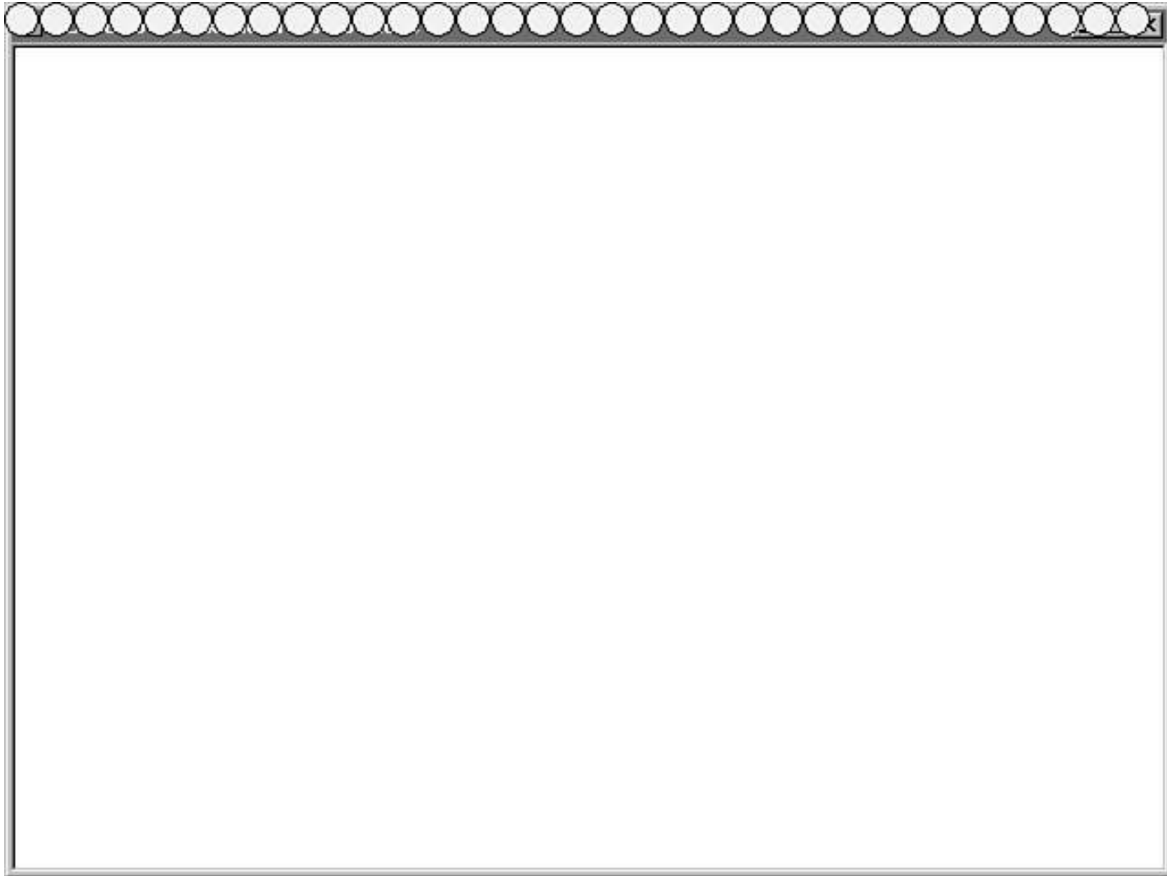
Figure 4.6 The series of circles across the main nonclient area results from successive calls to a CWindowDCobject 's Ellipse() method.
