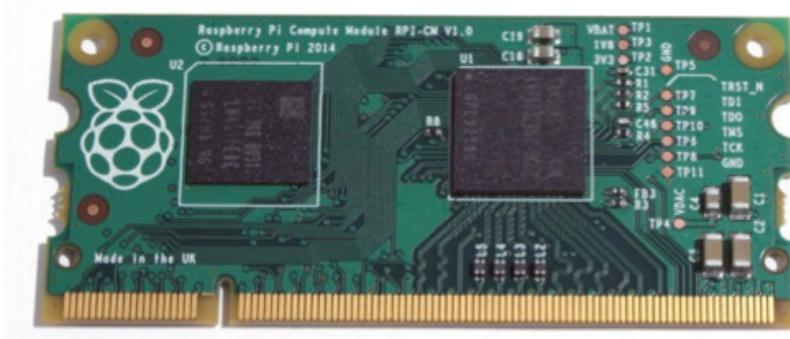
**Figura 4.14.** Placa Raspberry Pi Compute Module (<https://www.raspberrypi.org/blog/raspberrypi-compute-module-new-product>).
