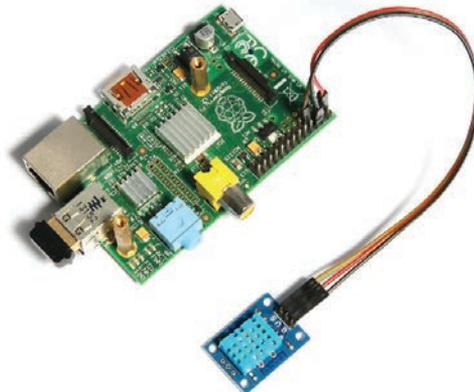
**Figura 8.28.** Raspberry Pi conectado con el sensor DHT11: <http://www.uugear.com/portfolio/dht11-humidity-temperature-sensor-module>.
