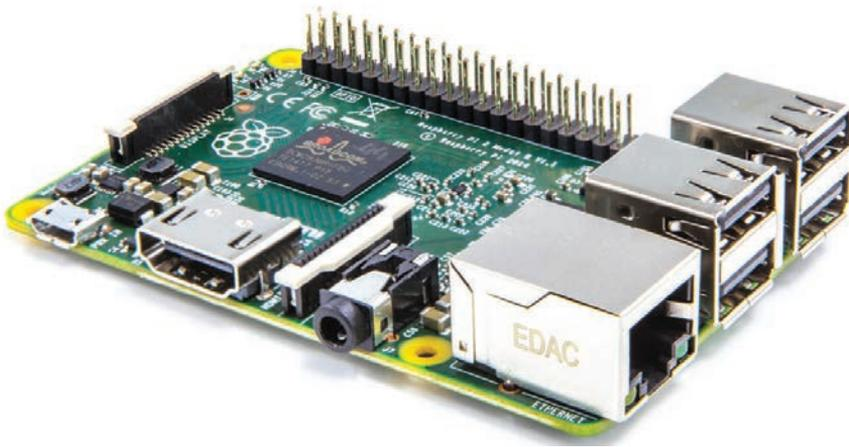
**Figura 4.7.** Placa Raspberry Pi 2 Modelo B (<http://www.zdnet.com/pictures/photos-of-the-raspberry-pi-through-the-ages-from-the-prototype-to-pi-3/7>).
