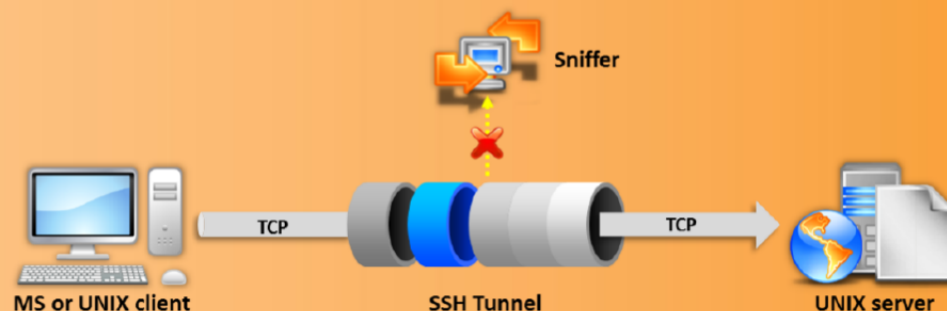
FIGURE 19.7: Secure shell tunneling
