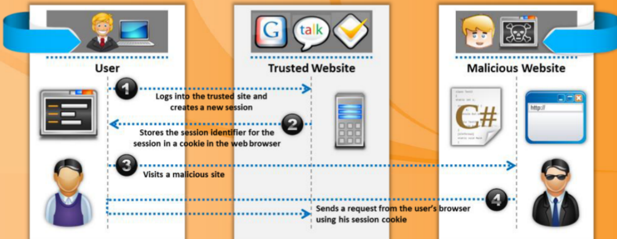
FIGURE 13.23: Cross-site Request Forgery (CSRF) Attack
