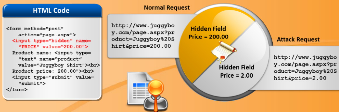
FIGURE 13.14: Hidden Field Manipulation Attack
