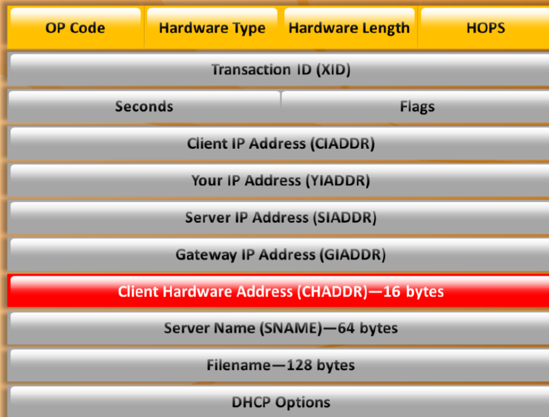
FIGURE 8.23: IPv4 DHCP Packet Format
