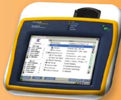
FIGURE 8.11: FLUKE Networks EtherScope™ Series II Network Assistant
