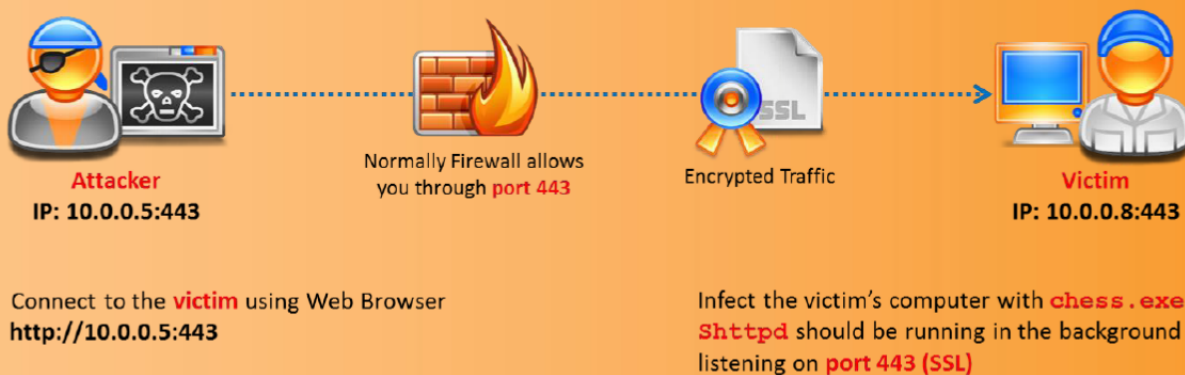
FIGURE 6.26: Attacker infecting Victim's system using Sshpd Trojan
