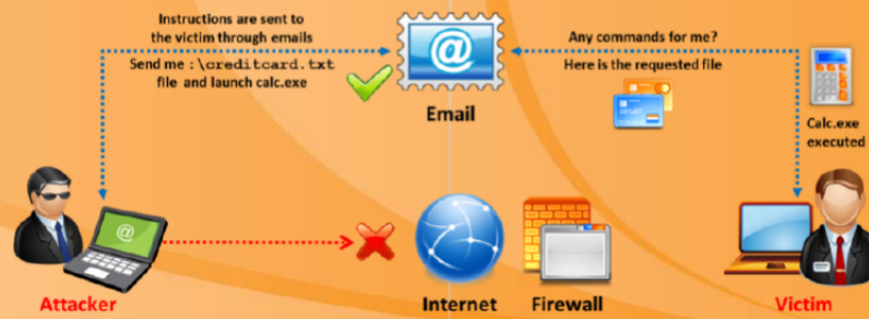
FIGURE 6.15: Illustrating the attack process using email Trojans
