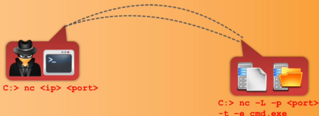
FIGURE 6.10: Attacker launching command shell Trojan in victim's machine
