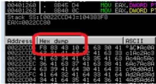
As the highlight section shows the correct information is loaded at the correct location on the stack. The program no longer crashes and can run to the end of the function to the RETN instruction shown here:
