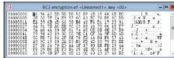
FIGURE 11.7: Output of RC2 - encrypted data
