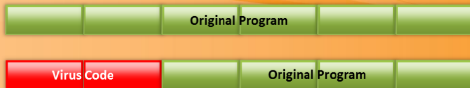
FIGURE 7.19: Working of Intrusive Viruses
