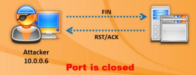
FIGURE 3.23: FIN Scan when Port is Closed
