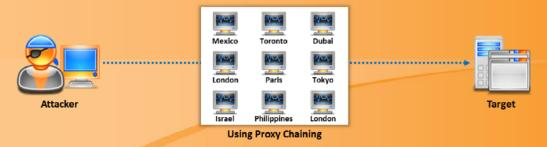
FIGURE 3.60: Attacker using Proxy Chaining for the attack
