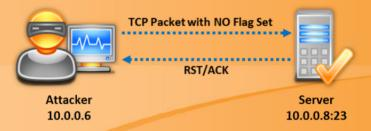
FIGURE 3.26: NULL Scan when Port is Closed
