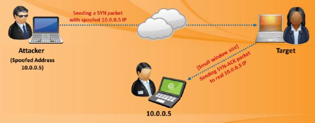
FIGURE 3.82: Using TCP Flow Control Method for IP Spoofing Detection
