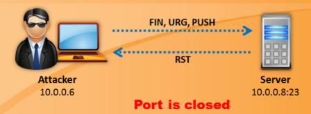
FIGURE 3.20: Xmas Scan when Port is Closed
