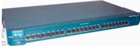
Figura 4.16. Switch catalyst de Cisco System
