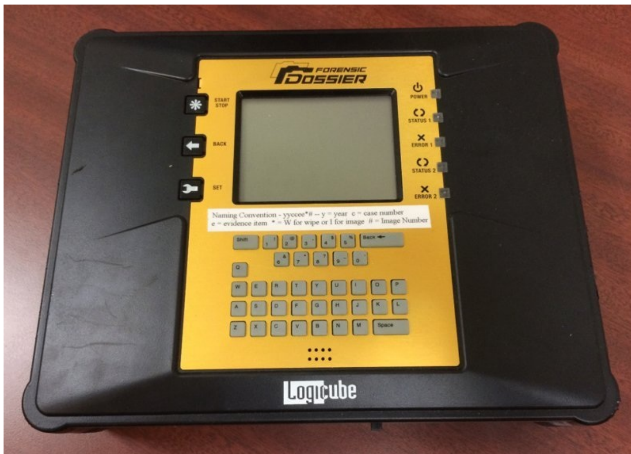
Figure 7.7 Logicube's Forensic Dossier duplicator device
