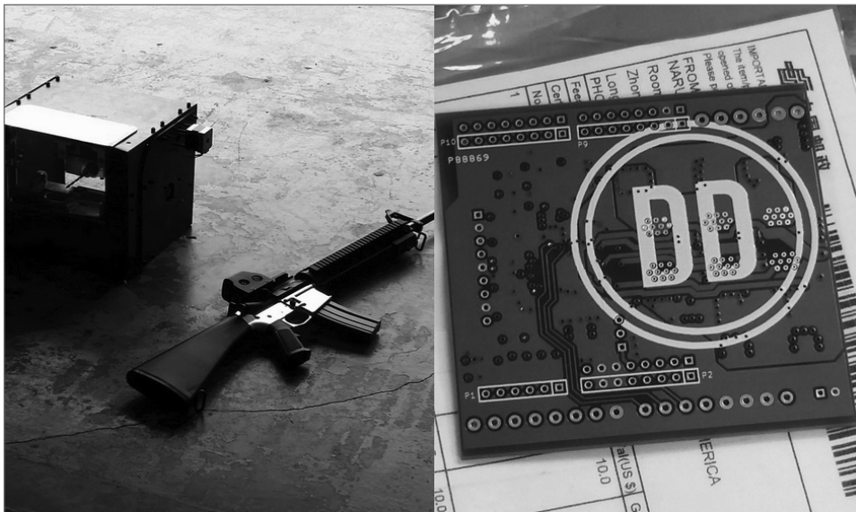
Figure 5-1: Defense distributed ghost gunner. An open source CNC machine designed to manufacture AR-15 lower receivers restricted under Federal law.
