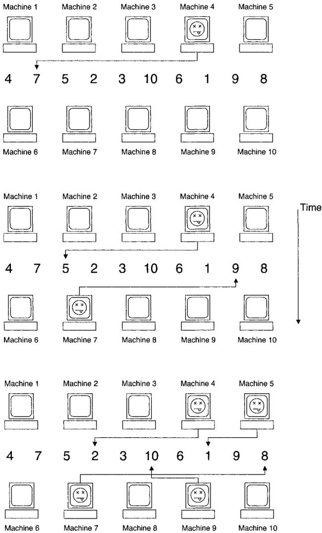
Figure 7.5. Permutation scanning
