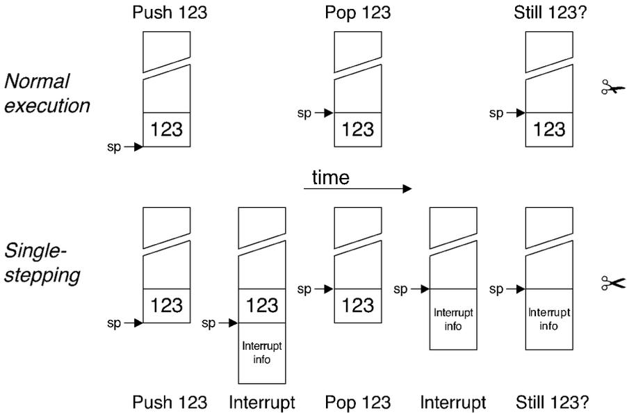
Figure 5.1. Checking for single-stepping
