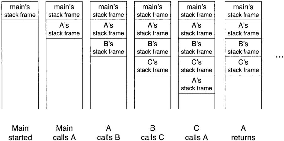
Figure 6.3. Stack frame trace
