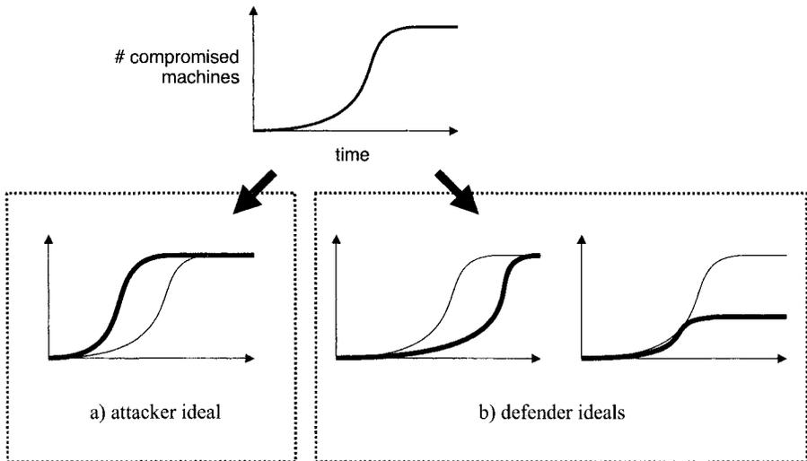
Figure 1.2. Ideal propagation curves for attackers and defenders
