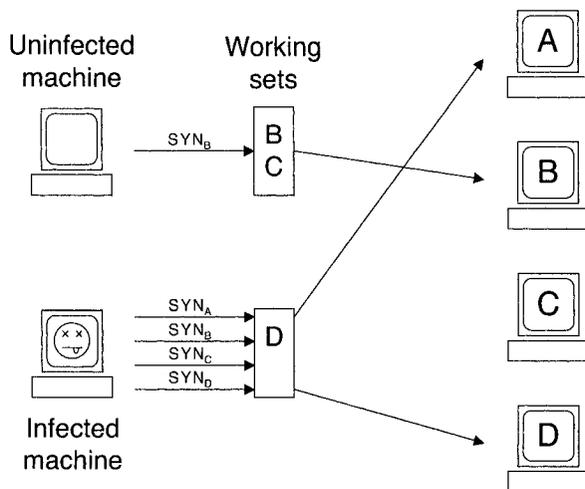
Figure 8.6. Network traffic throttling
