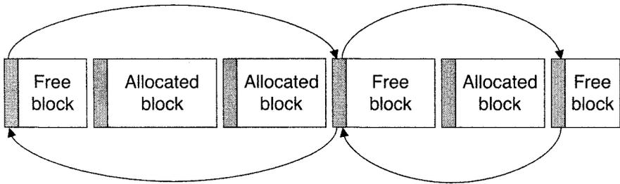
Figure 6.13. Dynamic memory allocator's free list
