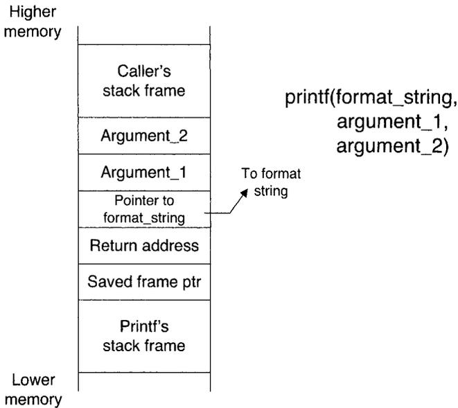
Figure 6.17. Stack layout for calling a format function
