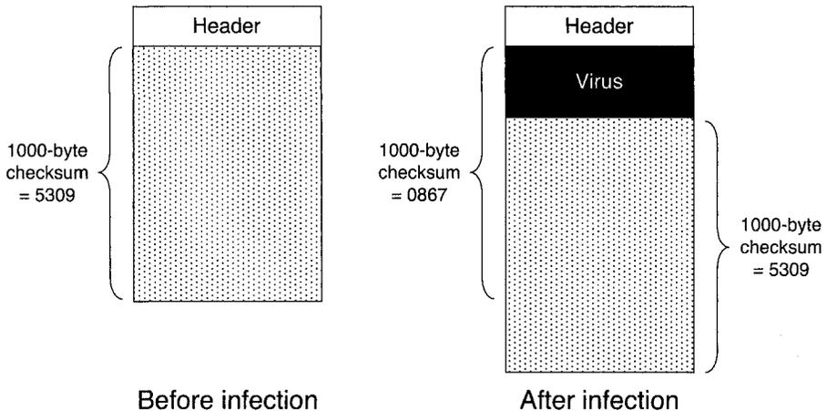
Figure 4.14. Disinfection using checksums
