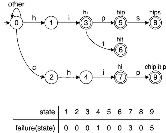
Figure 4.2. Aho-Corasick finite automaton and failure function
