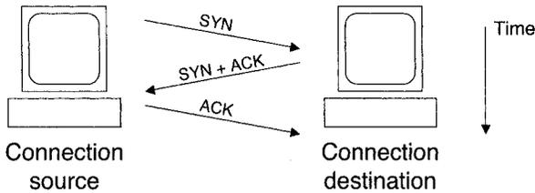
Figure 7.3. TCP connection establishment
