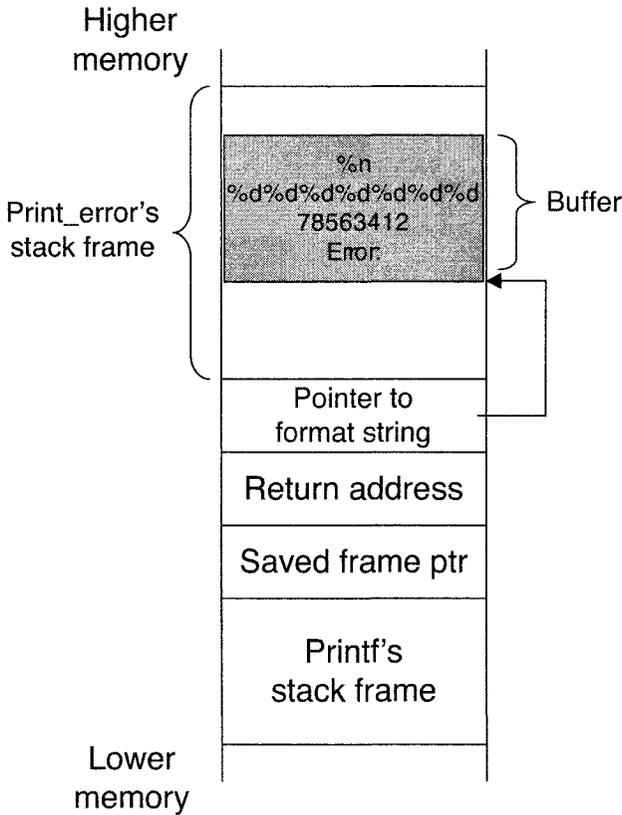
Figure 6.19. Format string attack in progress
