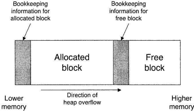
Figure 6.12. Overflowing the heap onto bookkeeping information
