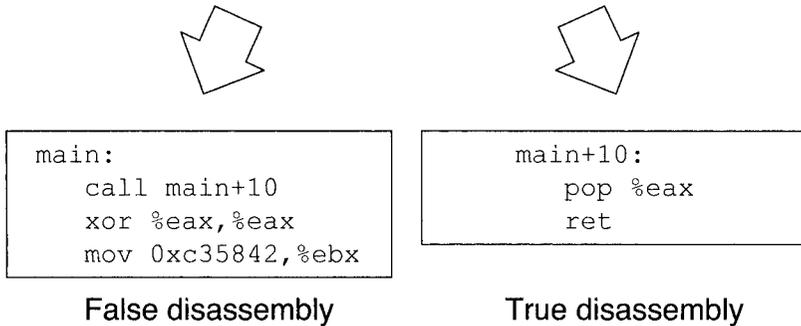
Figure 5.2. False disassembly
