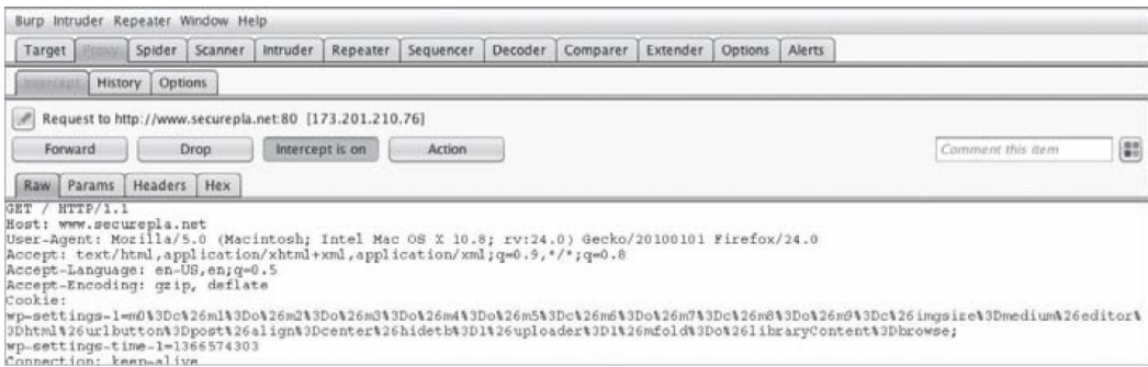
Figure 17 - Burp Capture and Intercepting Traffic
