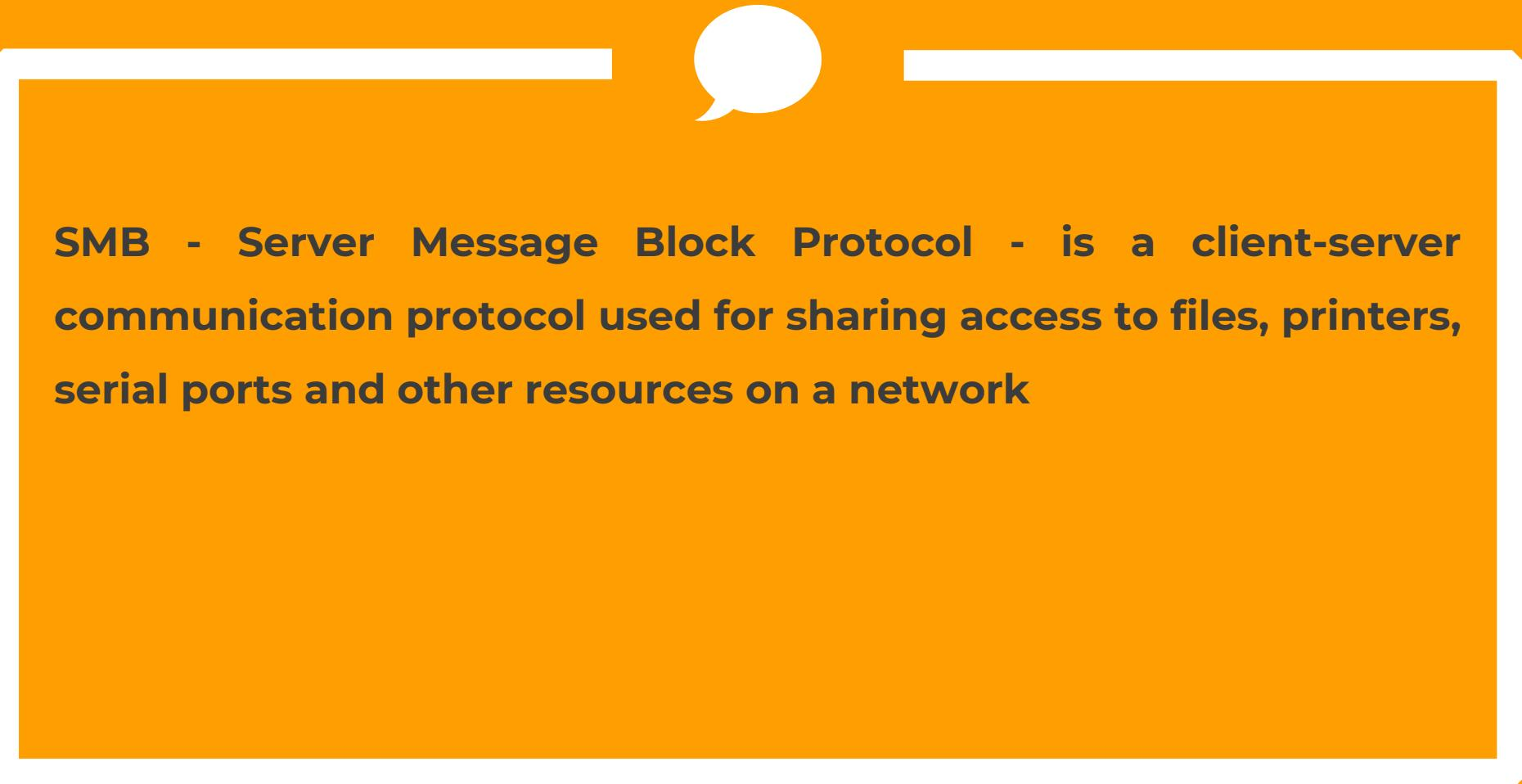
**SMB - Server Message Block Protocol - is a client-server communication protocol used for sharing access to files, printers, serial ports and other resources on a network**
