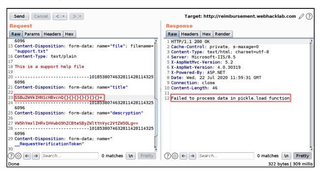
**Step 5:** Use the python script to generate a python deserialization payload using the script available in the Kali machine to receive an out-of-band call as shown below:
