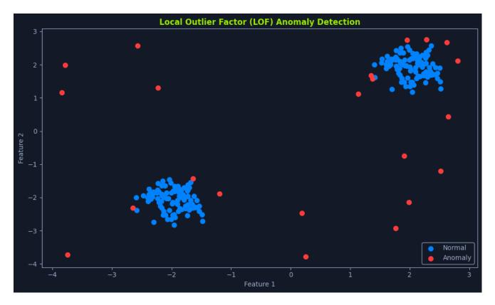
Local Outlier Factor (LOF) is a density-based algorithm designed to identify outliers in datasets by comparing the local density of a data point to that of its neighbors. It is particularly effective in detecting anomalies in regions where the density of points varies significantly.
