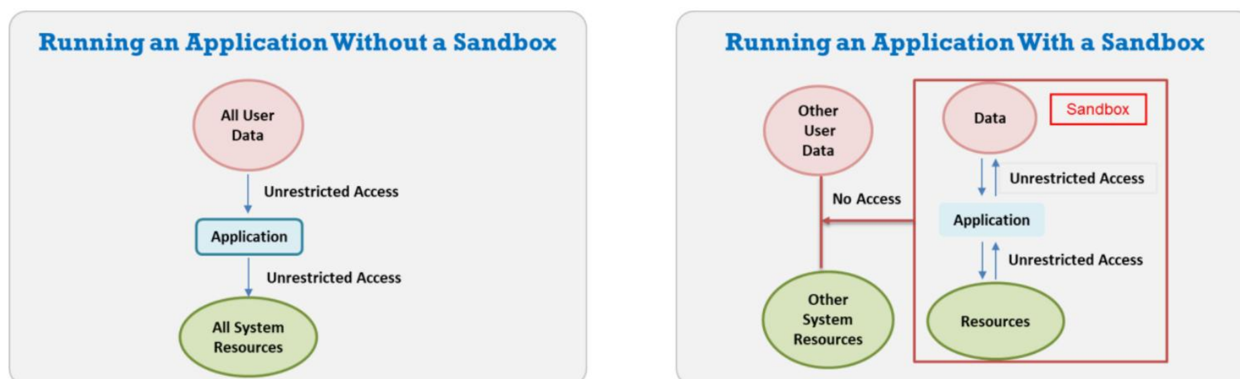
Figure 9.25: Execution of an application with and without a sandbox
