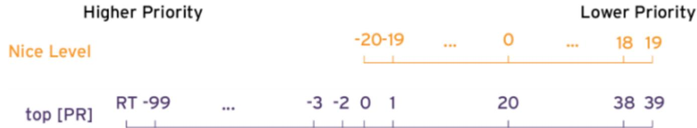
Nice value is a user-space and priority PR is the process's actual priority that use by Linux kernel. In Linux system priorities are 0 to 139 in which 0 to 99 for real time and 100 to 139 for users
