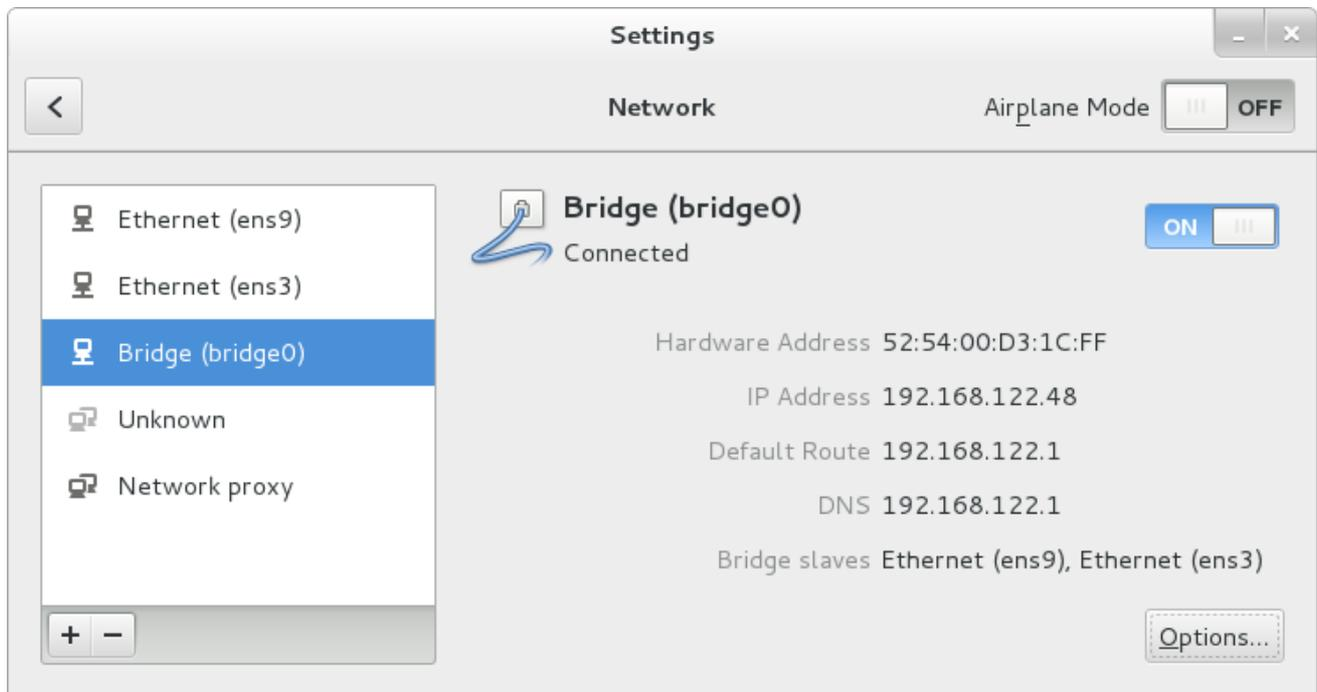
Figure 6.8. The NetworkManager Graphical User Interface with Bridge
