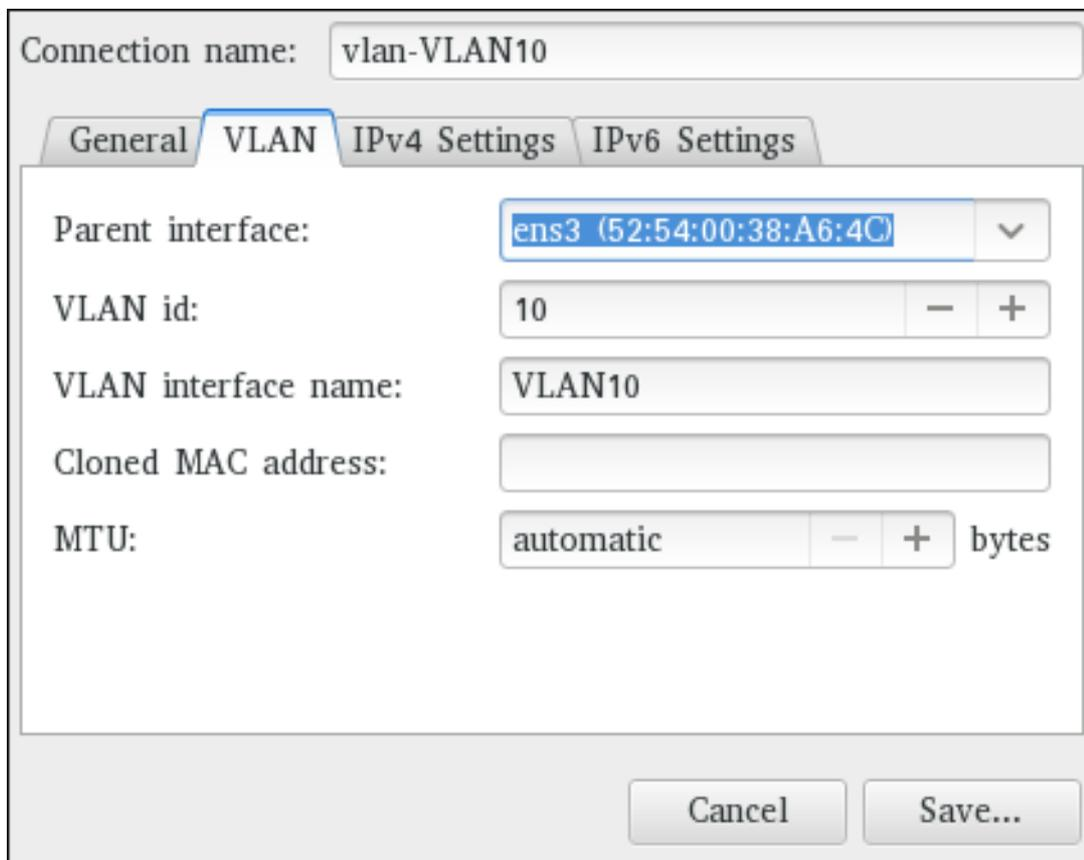
Figure 7.3. Adding a New VLAN Connection Using nm-connection-editor
