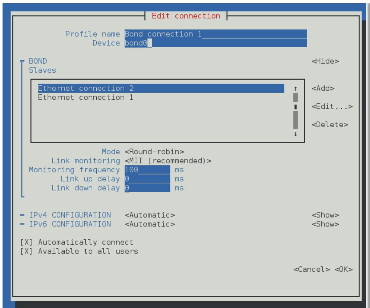
Figure 4.5. The NetworkManager Text User Interface Completed Bond
