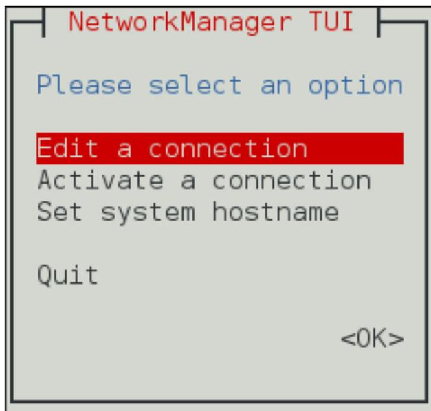
Figure 3.1. The NetworkManager Text User Interface starting menu
