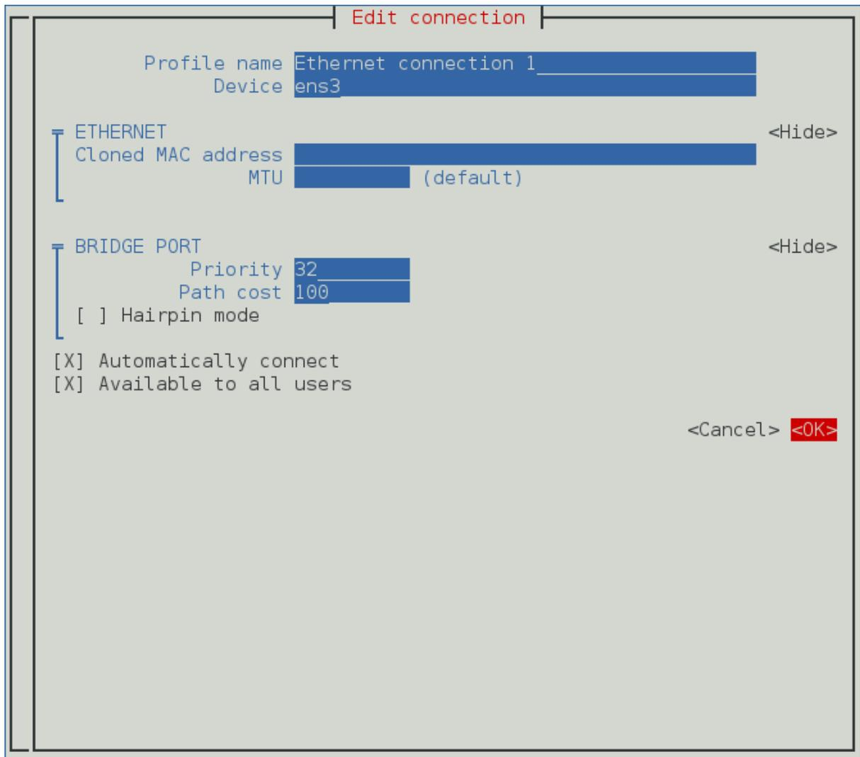
**Figure 6.3. The NetworkManager Text User Interface Configuring a Bridge Slave Connection menu**
