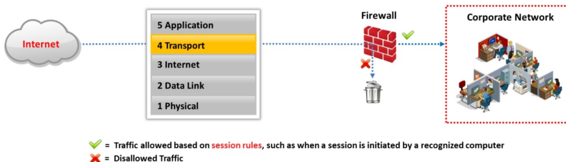
Figure 12.14 Example of Circuit-Level Gateway Firewall
