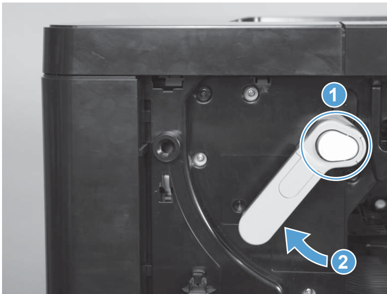
Figure 1-304 Remove the drive assembly (M830; 1 of 3)
