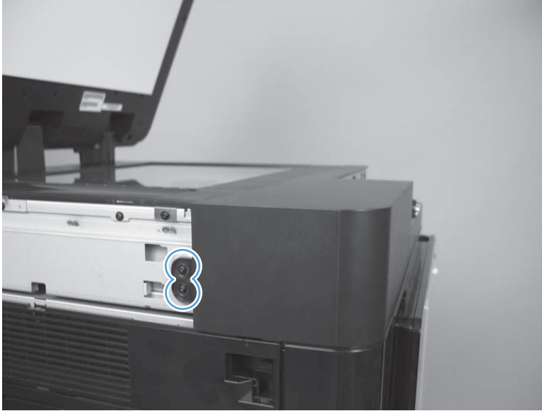
Figure 1-121 Remove the scanner front cover (M830; 4 of 7)
