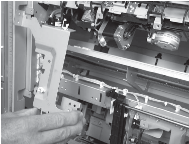
Figure 1-621 Remove the paper face sensor and flag assembly (9 of 9)
