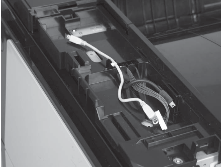
Figure 1-143 Reinstall the control-panel base cover (M806; 1 of 3)
