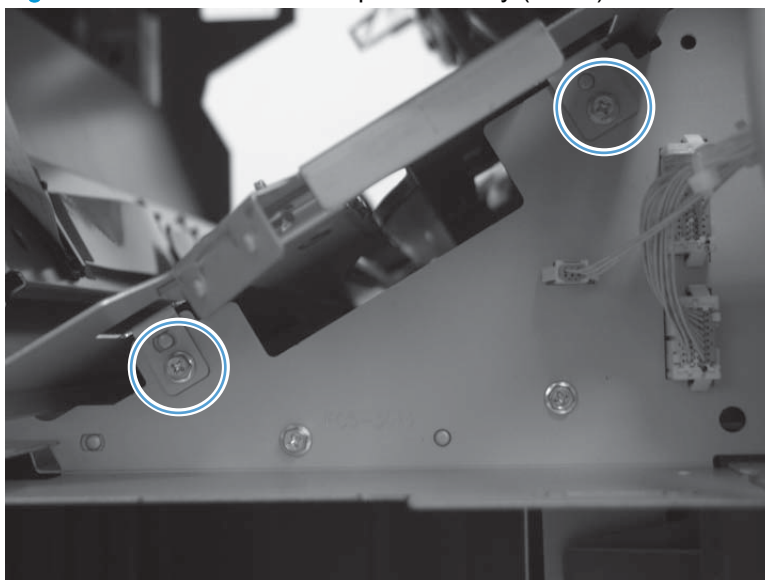
Figure 1-630 Remove the staple assembly (1 of 7)
