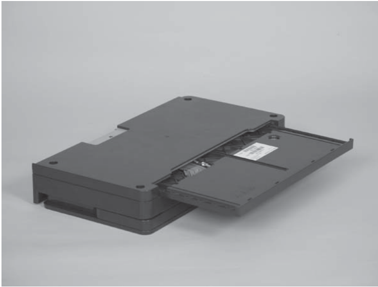
Figure 1-75 Remove the keyboard assembly (M830; 6 of 7)
