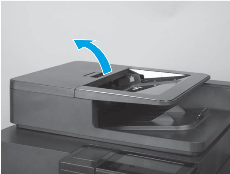
Figure 1-84 Remove the document-feeder roller (M830; 1 of 3)
