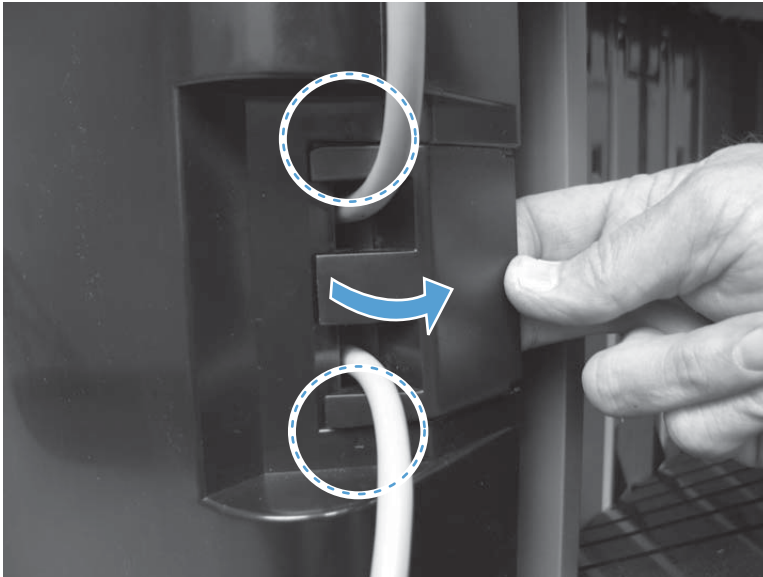
Figure 1-479 Remove the bin cable guide cover (3 of 6)
