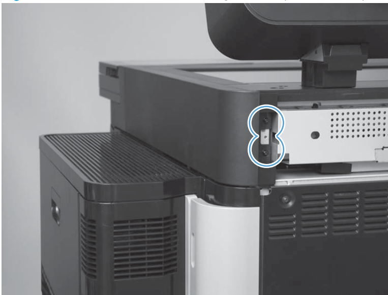
Figure 1-115 Remove the scanner right cover (M830; 2 of 4)
