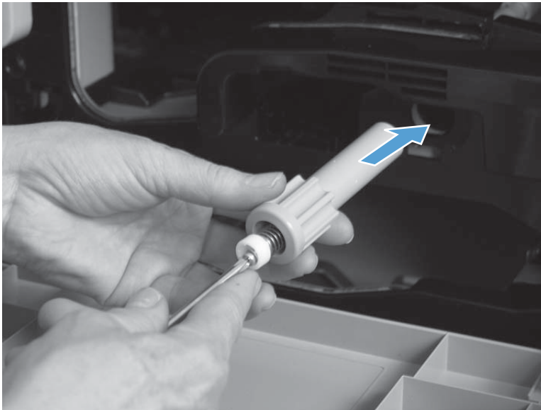
Figure 1-232 Reinstall the registration-jam-removal knob (2 of 3)
