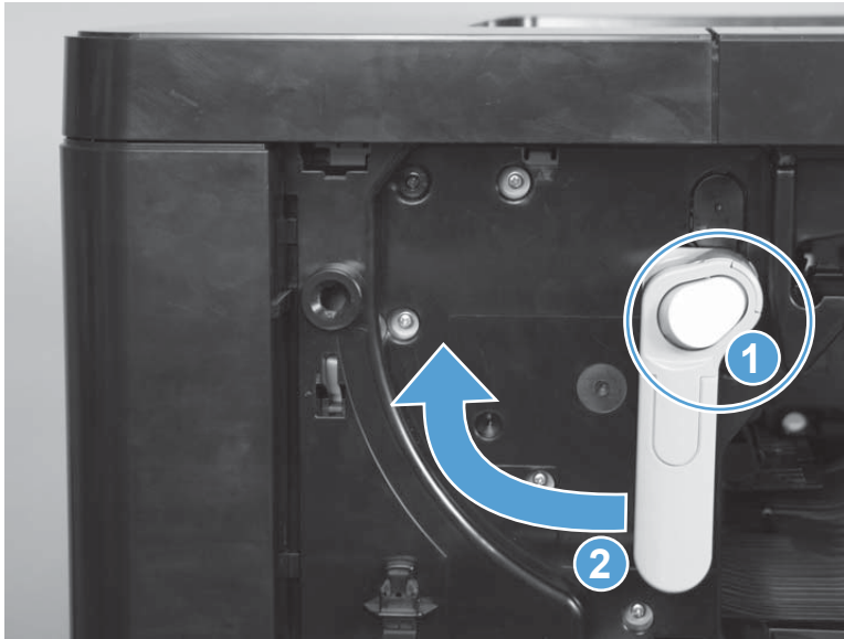
Figure 1-5 Reinstall the toner cartridge
