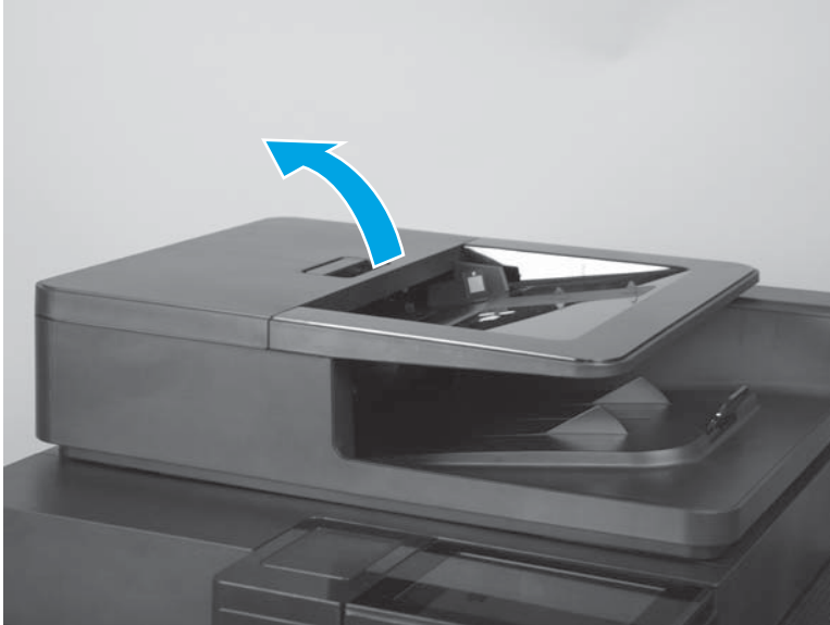
Figure 1-88 Remove the document-feeder separation pad (M830; 1 of 4)
