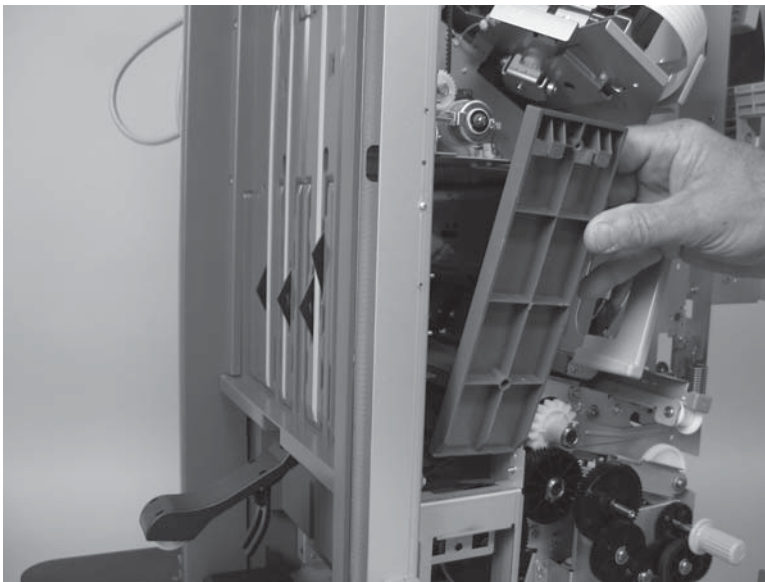
Figure 1-771 Remove the saddle delivery inner cover, front assembly (3 of 3)
