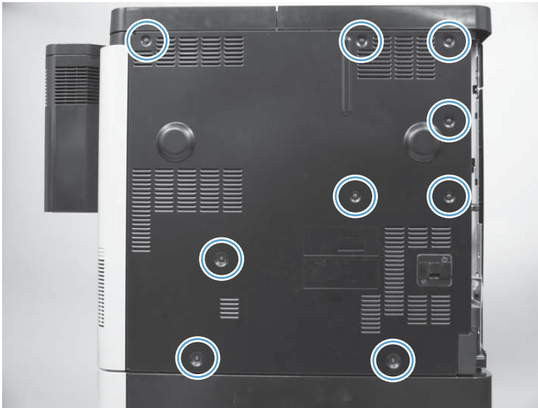
Figure 1-166 Remove the rear cover (2 of 3)
