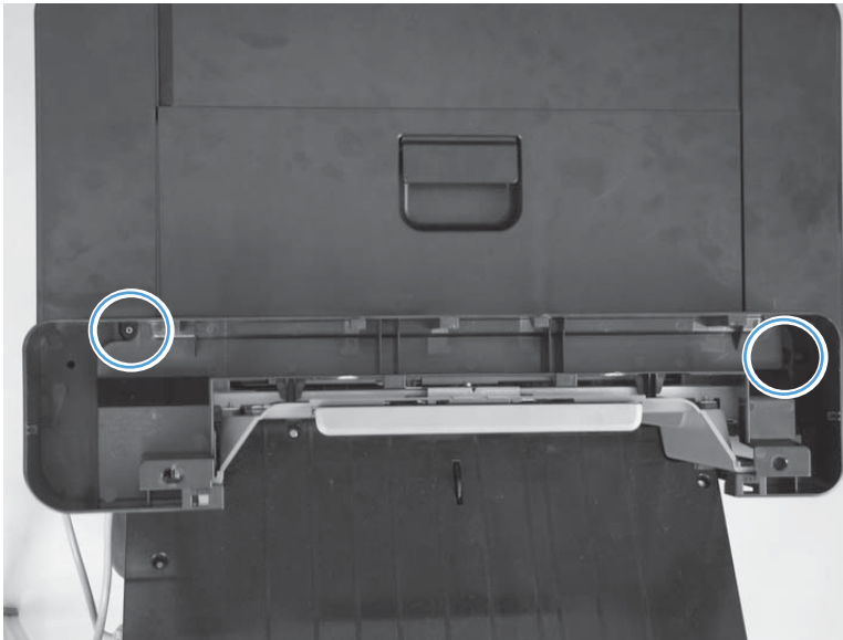
Figure 1-491 Remove the lower stepped cover assembly (1 of 5)
