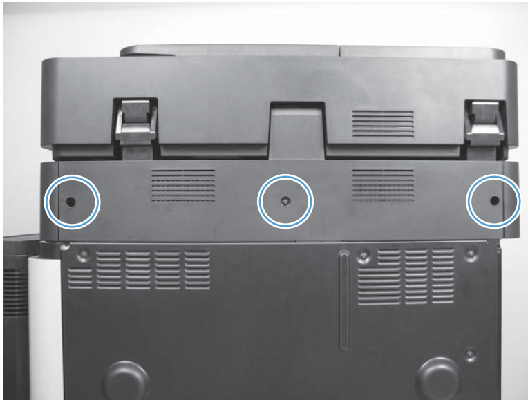
Figure 1-109 Remove the scanner back cover (M830; 1 of 2)
