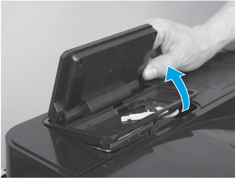
Figure 1-53 Remove the control-panel assembly (M806; 5 of 10)
