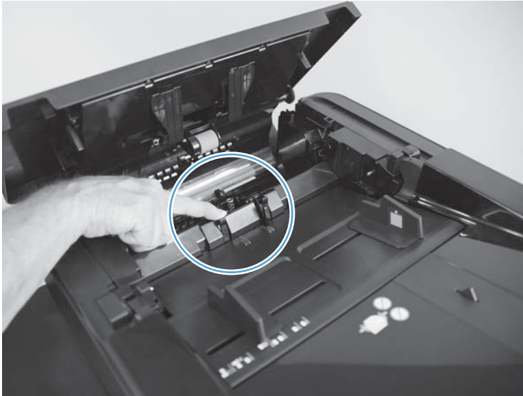
Figure 1-92 Reinstall the document-feeder separation pad (M830; 1 of 5)
