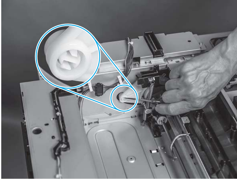
Figure 1-345 Remove the cartridge-lifter assembly (M830; 12 of 14)
