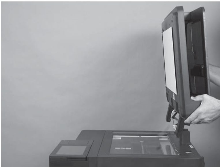
Figure 1-217 Remove the document feeder assembly (M830; 7 of 7)
