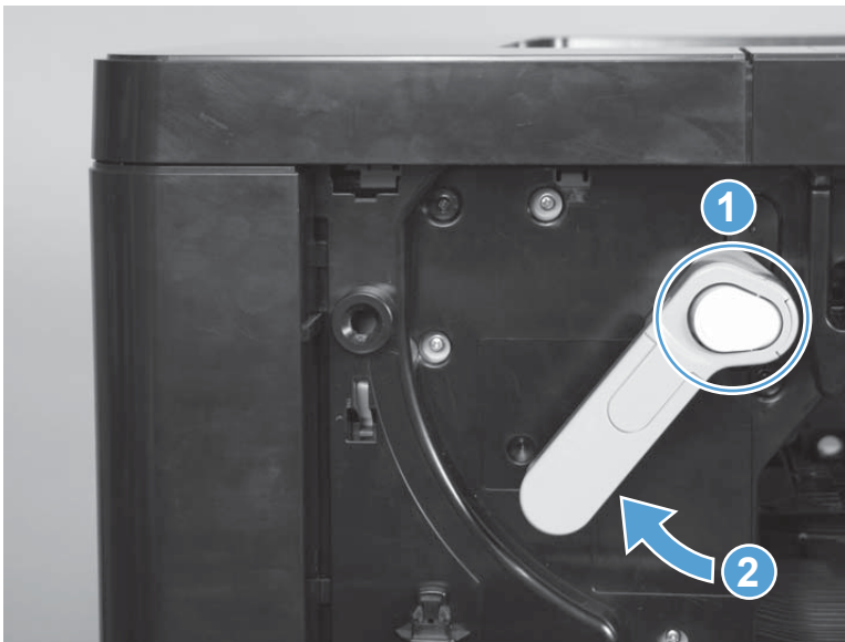
Figure 1-299 Remove the drive assembly (M806; 1 of 3)
