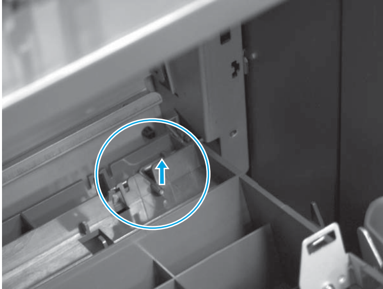
Figure 1-813 Remove the saddle paper delivery assembly (6 of 8)
