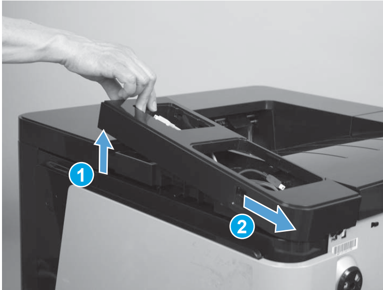
Figure 1-142 Remove the control-panel base cover (M806; 3 of 3)
