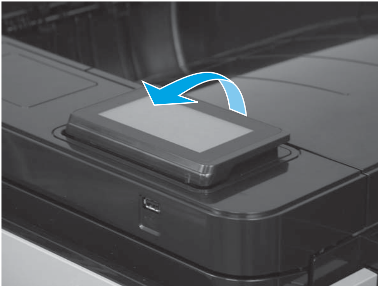
Figure 1-49 Remove the control-panel assembly (M806; 1 of 10)
