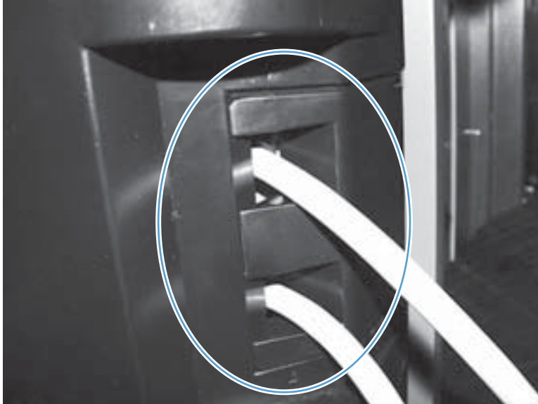
Figure 1-484 Bin cable guide cover incorrectly installed
