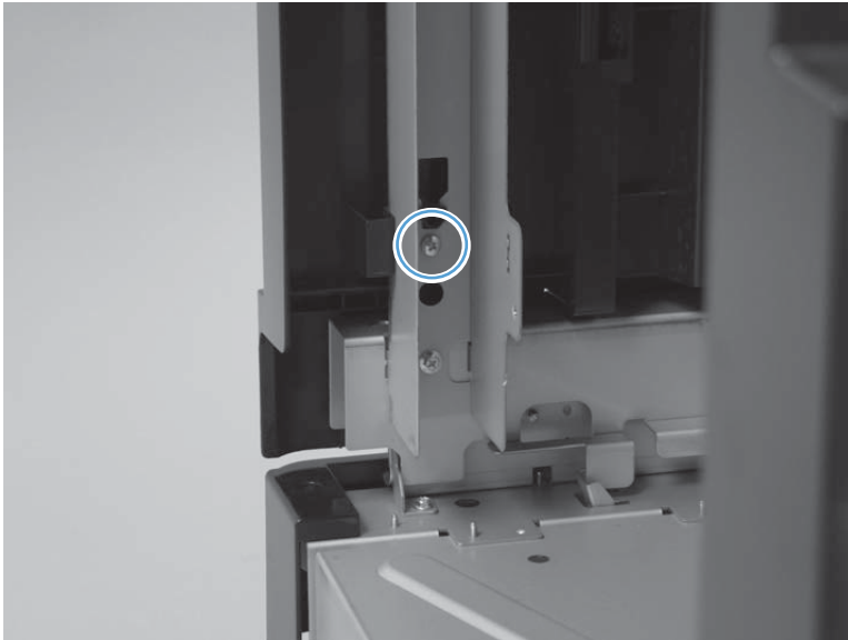
Figure 1-470 Remove the pre-reverse cover assembly (2 of 3)
