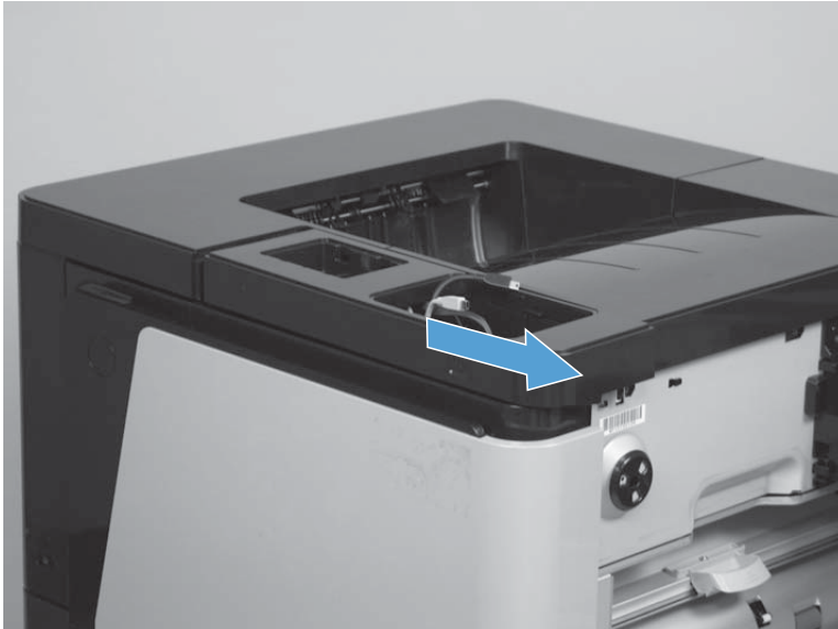
Figure 1-141 Remove the control-panel base cover (M806; 2 of 3)
