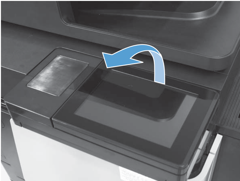
Figure 1-60 Remove the control-panel assembly (M830; 1 of 7)
