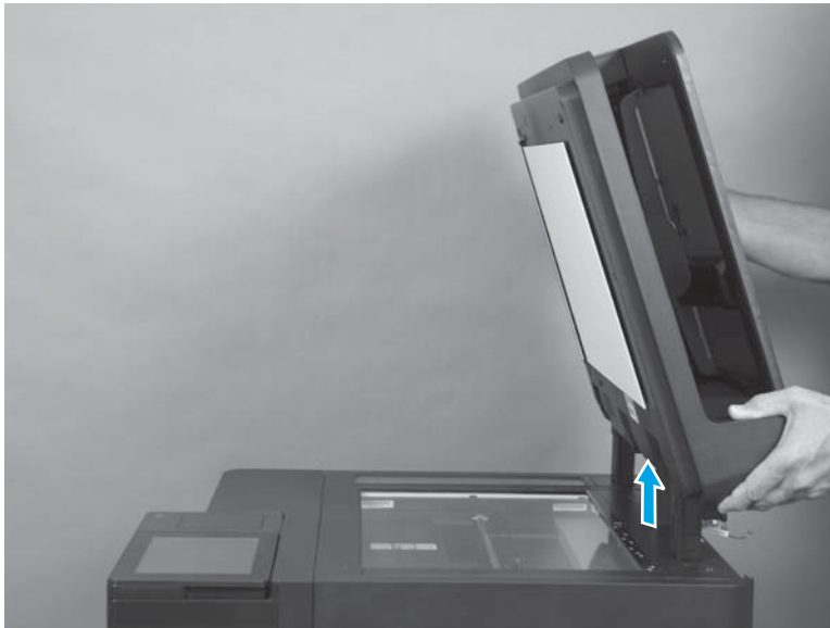
Figure 1-215 Remove the document feeder assembly (M830; 5 of 7)
