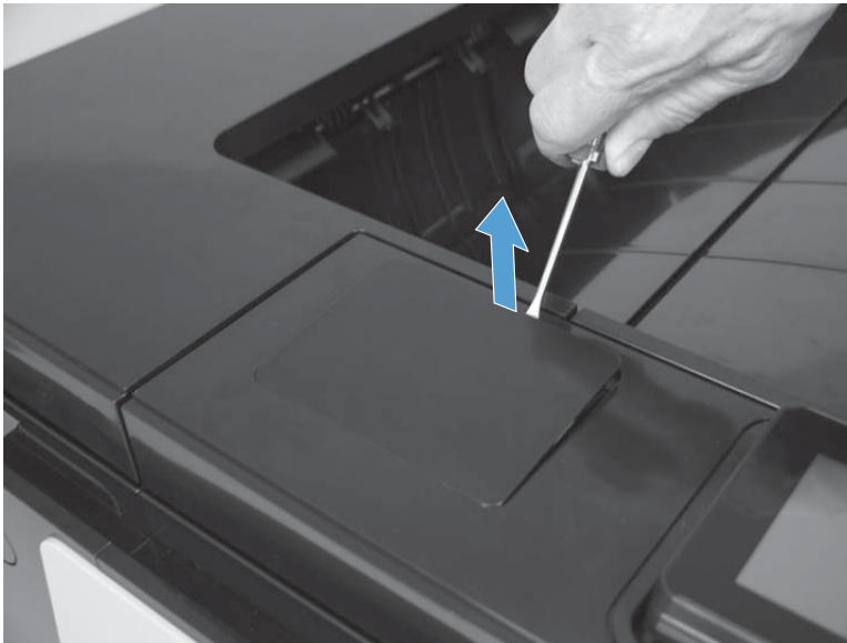
Figure 1-131 Remove the HIP cover (M806; 2 of 3)
