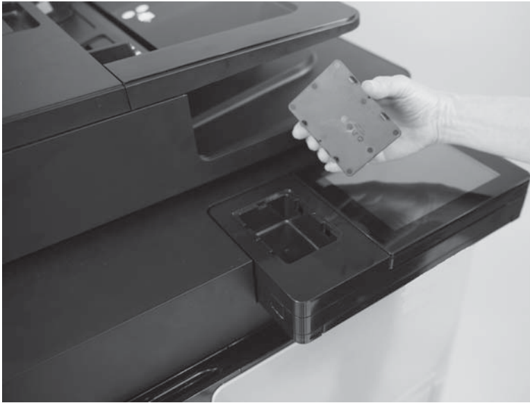
Figure 1-137 Remove the HIP cover (M830; 3 of 3)
