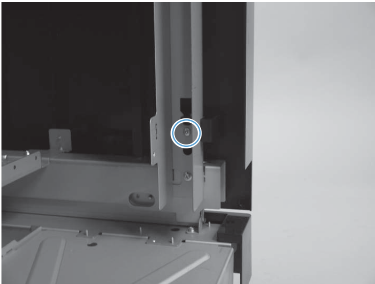
Figure 1-473 Remove the rear reverse cover assembly (2 of 3)
