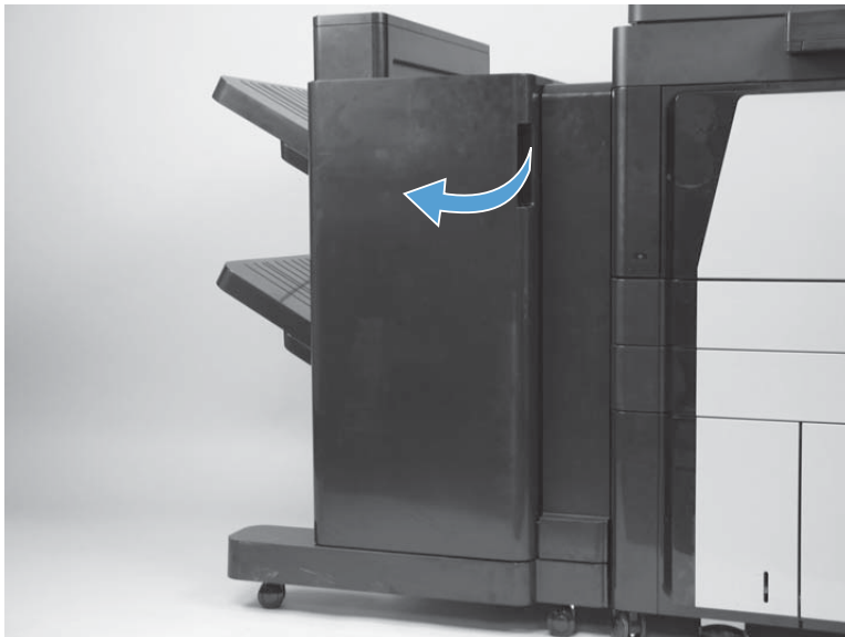
Figure 1-459 Disconnect a finishing accessory from the product (2 of 4)
