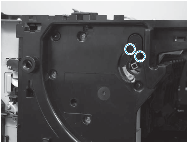
Figure 1-321 Remove the cartridge-lifter assembly (M806; 5 of 11)
