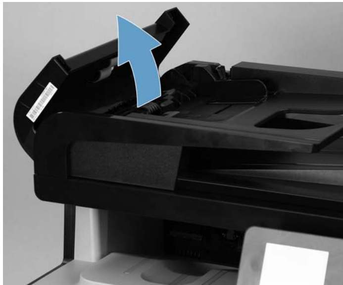
Figure 1-8 Open the jam-access cover
