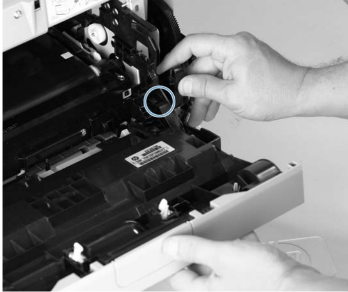
Figure 1-66 Remove the front-door assembly (6 of 10)
