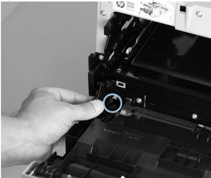
Figure 1-69 Remove the front-door assembly (9 of 10)
