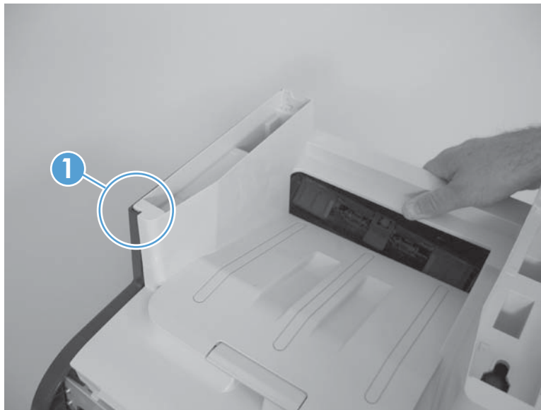
Figure 1-53 Reinstall the upper-cover assembly (1 of 3)
