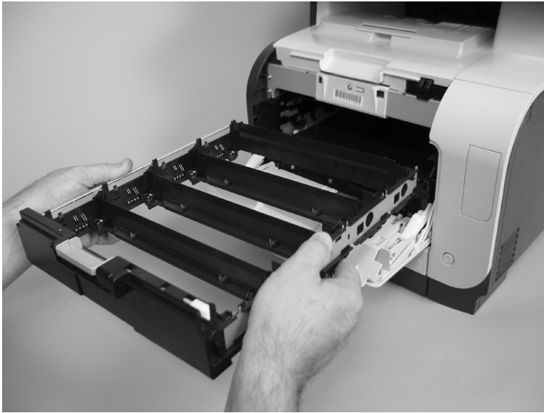
Figure 1-25 Remove the print-cartridge drawer (3 of 3)
