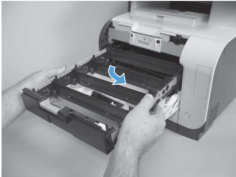
Figure 1-24 Remove the print-cartridge drawer (2 of 3)
