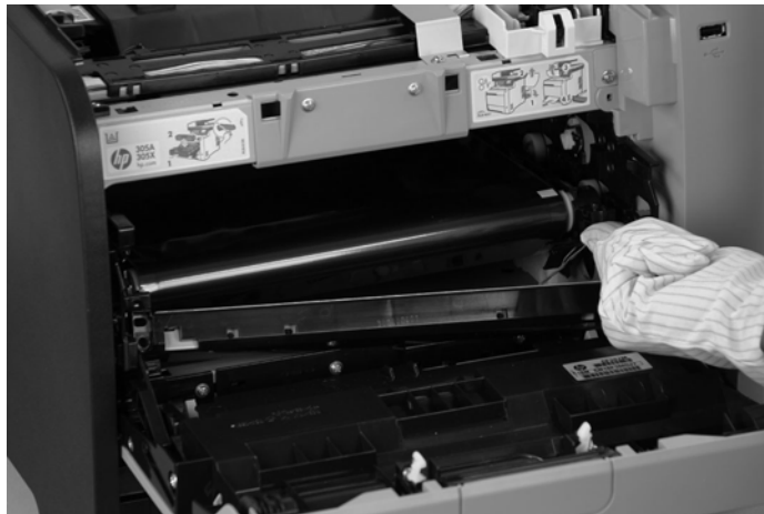
Figure 1-74 Remove the ITB (4 of 6)
