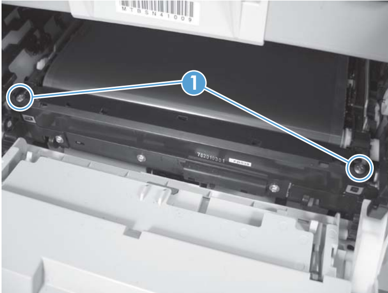
Figure 1-71 Remove the ITB (1 of 6)
