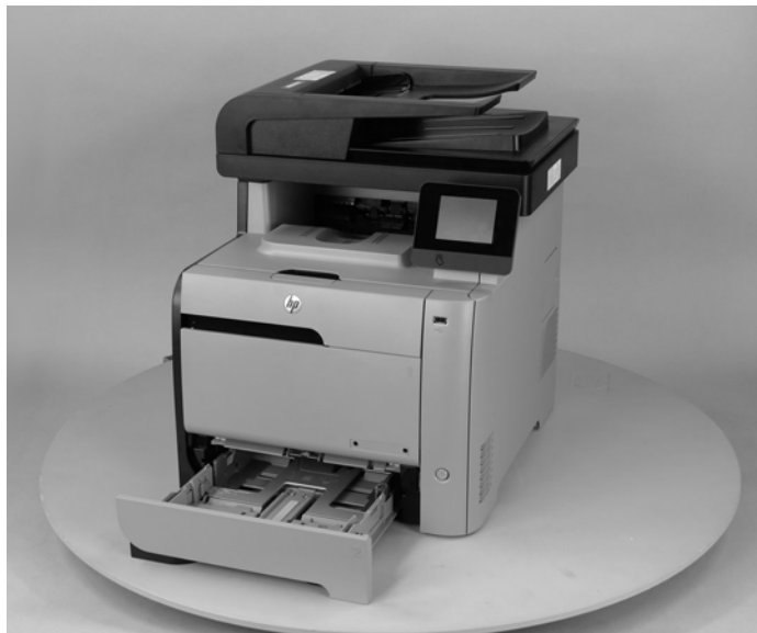
Figure 1-148 Remove the tray cassettes and optional Tray 3 assembly (1 of 2)
