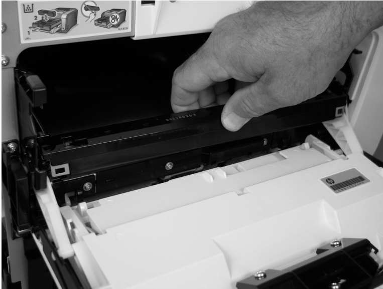
Figure 1-108 Remove the color-misregistration sensor assembly PCA (4 of 4)
