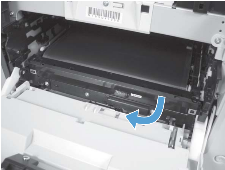
Figure 1-72 Remove the ITB (2 of 6)
