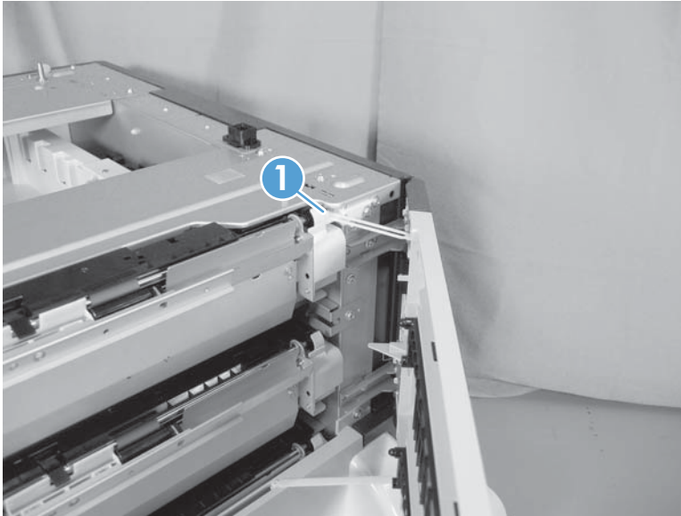
Figure 2-201 Remove the 3 x 500 right-door assembly (1 of 3)
