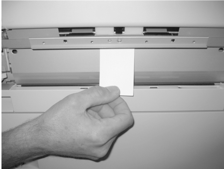
Figure 3-21 Test the Tray 3 feed sensor
