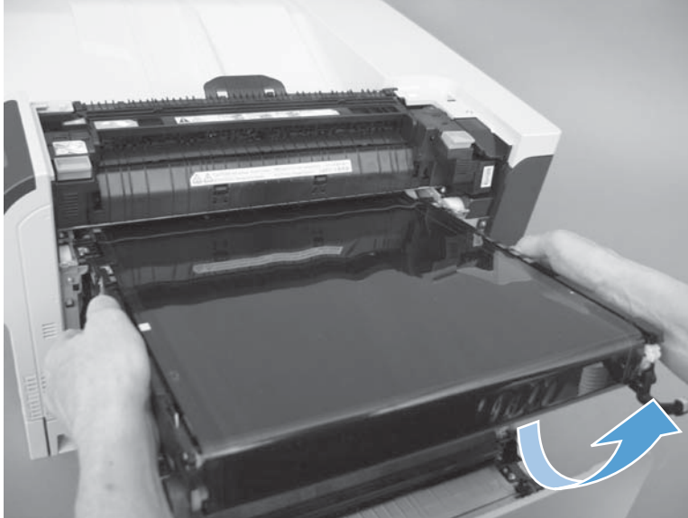
Figure 2-20 Remove the intermediate transfer belt (3 of 3)
