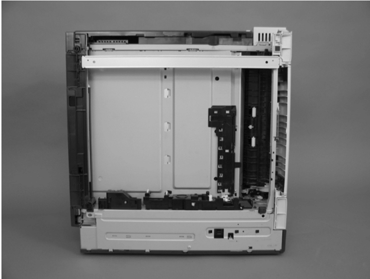
Figure 2-70 Remove the lifter-drive assembly (1 of 3)
