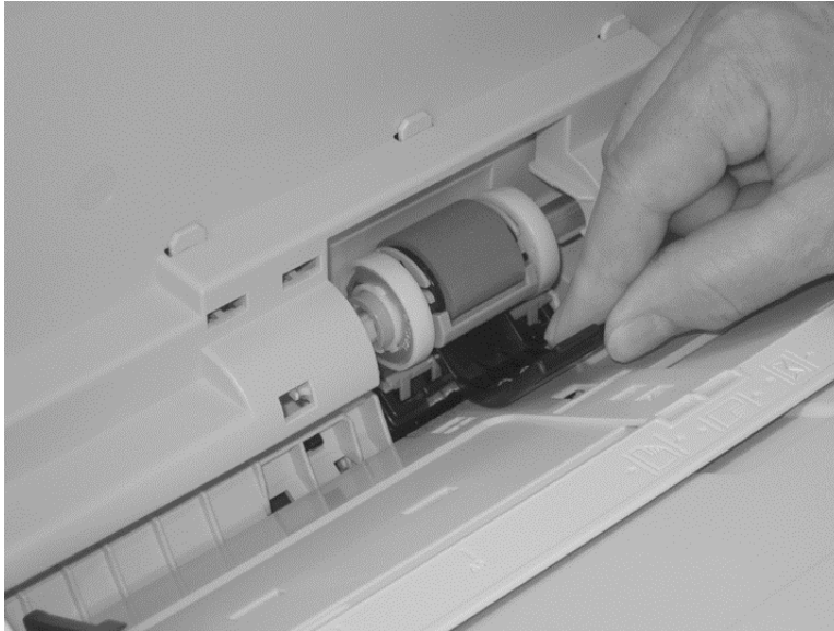
Figure 2-11 Remove the separation pad (Tray 1) (4 of 4)
