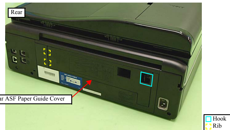
Figure 4-25. Removing the Rear ASF Paper Guide Cover
