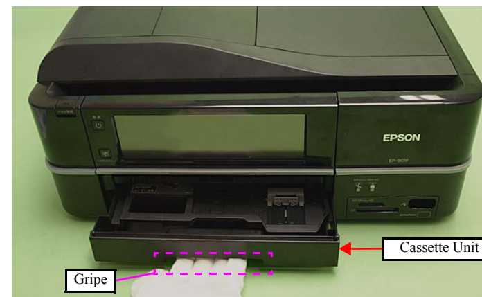
Figure 4-32. Removing the Cassette Unit
