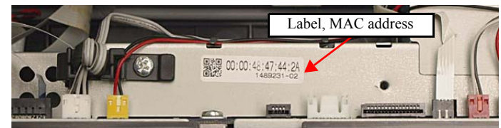
Figure 4-48. Position for the MAC Address Label
