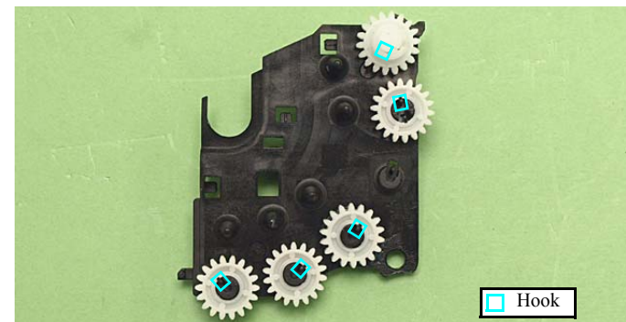
Figure 4-141. Installing the Transmission Holder Assy (1)
