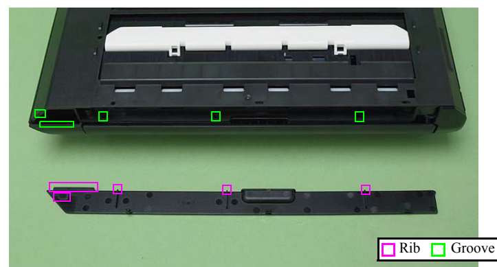
Figure 4-181. Installing the ADF Cover L
