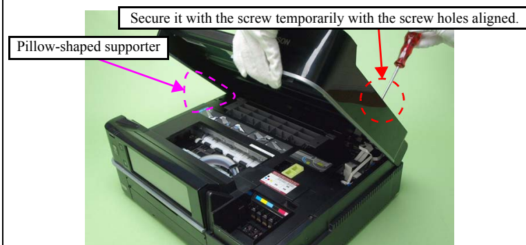
Figure 4-10. Installing the Scanner Unit (2)
