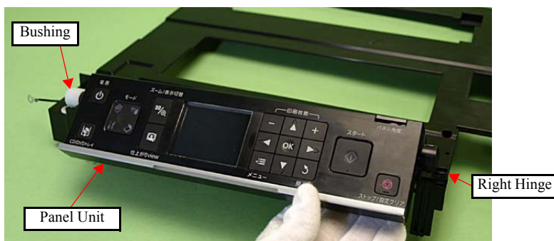
Figure 4-228. Removing the Panel Unit (3)
