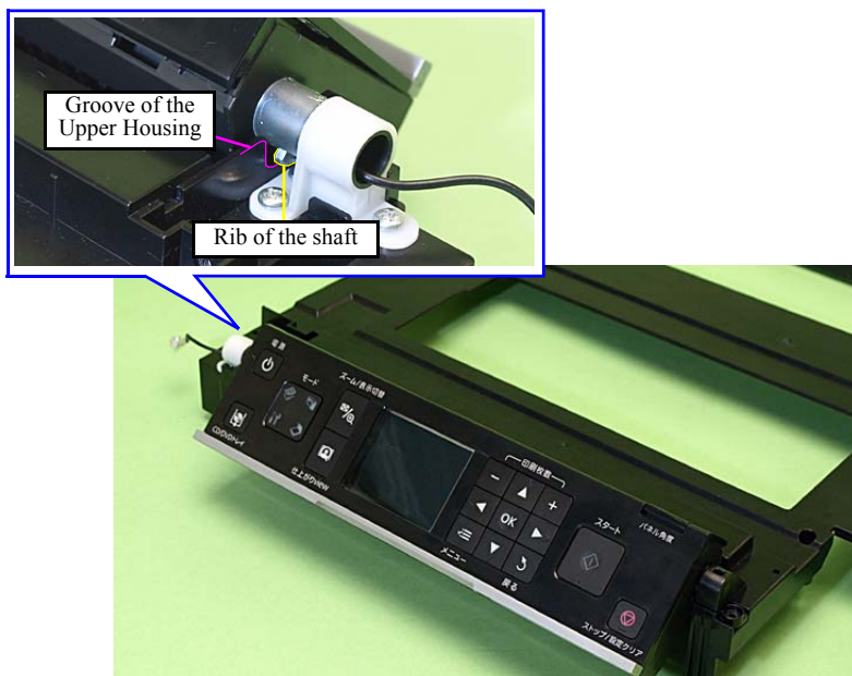
Figure 4-227. Removing the Panel Unit (2)
