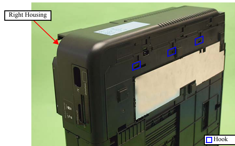
Figure 4-29. Removing the Right Housing/Card Cover (2)
