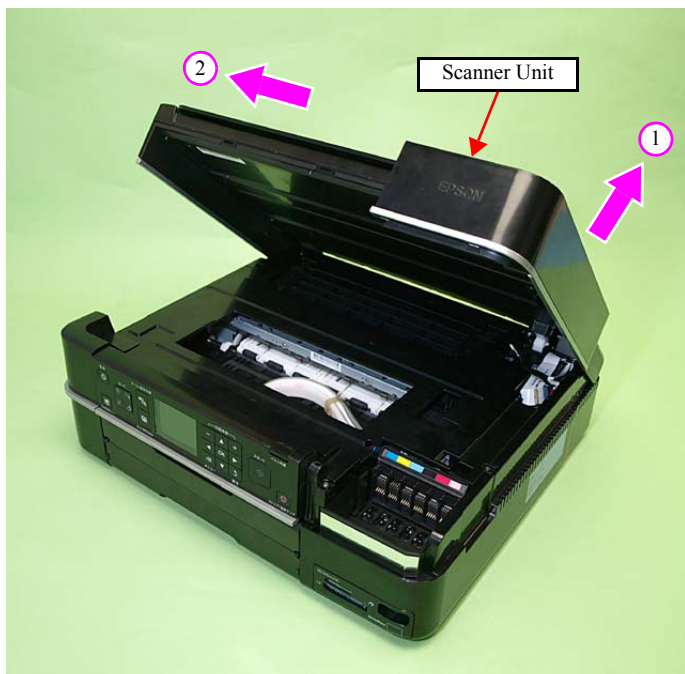
Figure 4-206. Removing the Scanner Unit (3)
