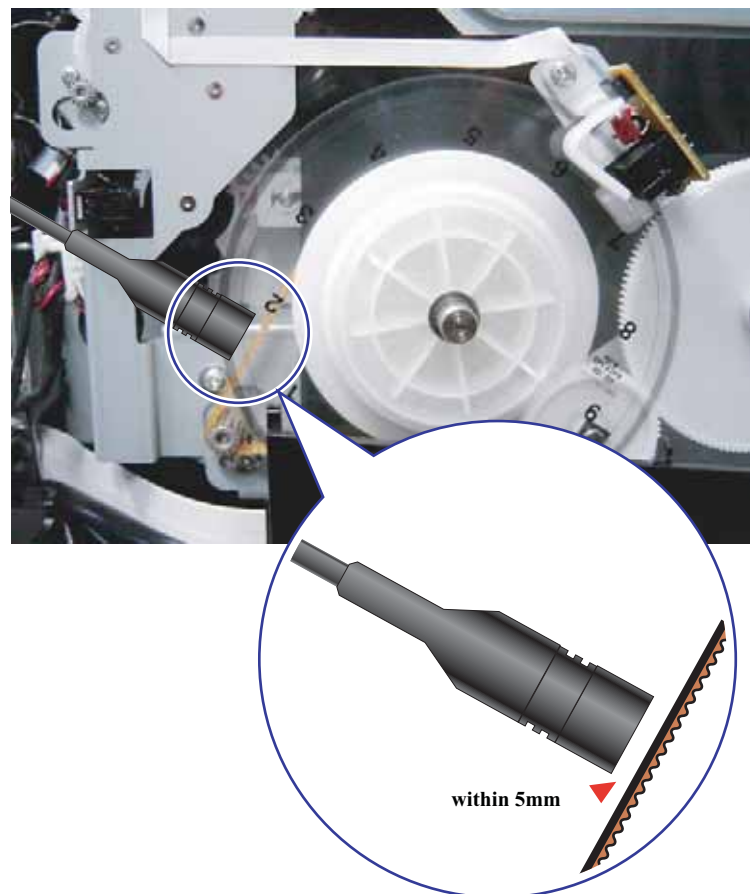
Figure 5-4. Tension Measurement
