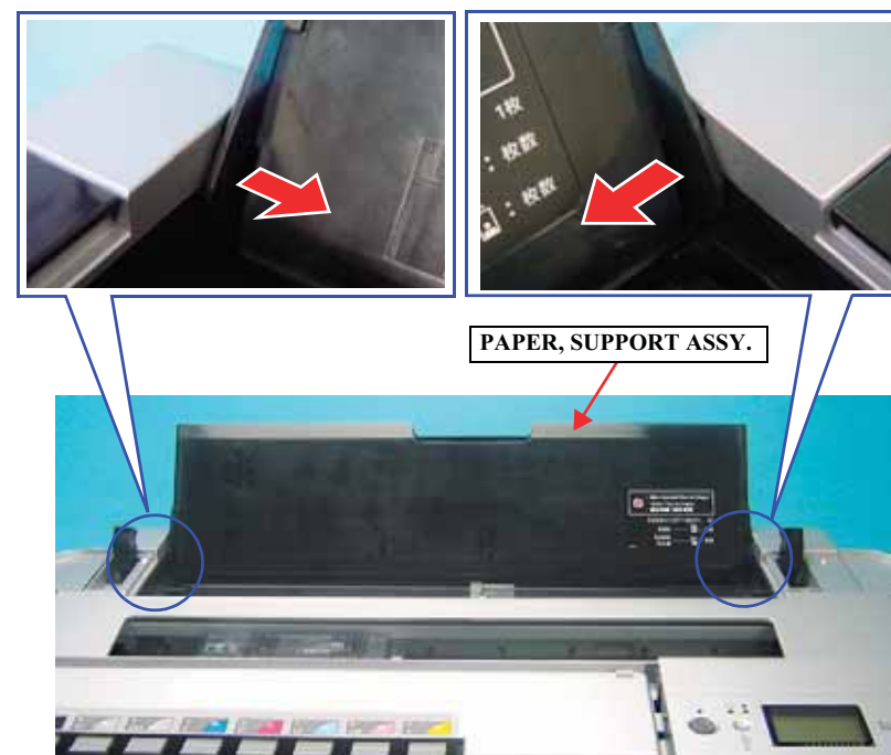
Figure 4-13. Removing the PAPER SUPPORT ASSY.
