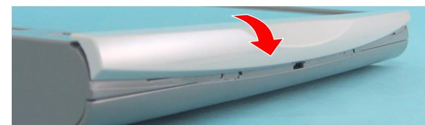
Figure 4-48. Installing Scanner Housing, Front
