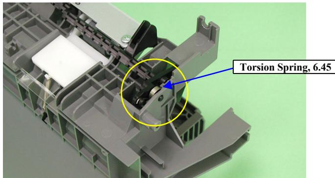
Figure 2-8. Torsion Springs, 6.45 installation
