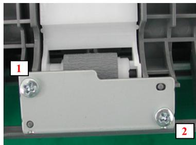
Figure 2-9. Support Plate, Frame, ASF installation
