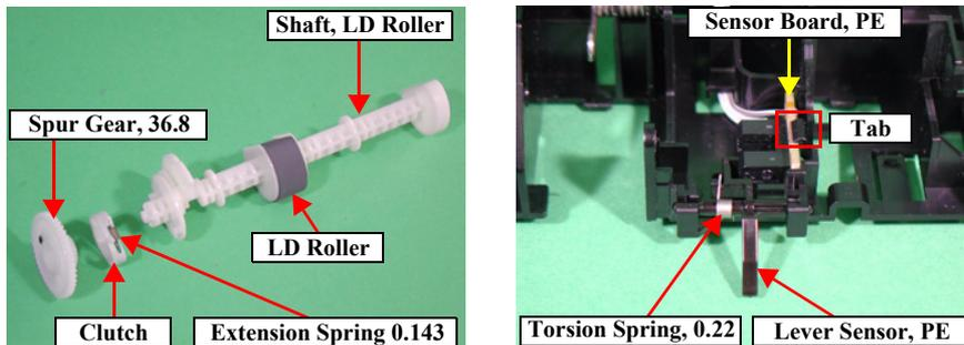
Figure 2-17. Holder, Shaft Assy. Removal (2)
