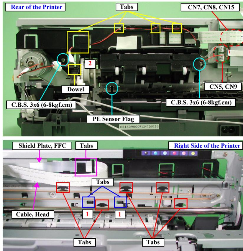
Figure 2-16. Holder, Shaft Assy. Removal (1)
