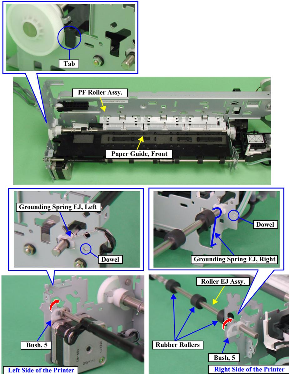
Figure 2-45. Paper Guide, Front/Roller EJ Assy. Removal (2)
