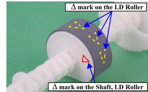
Figure 2-18. Reinstalling the LD Roller
