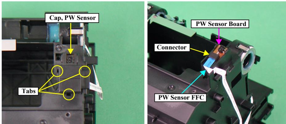
Figure 2-27. Carriage Unit Removal (2)
