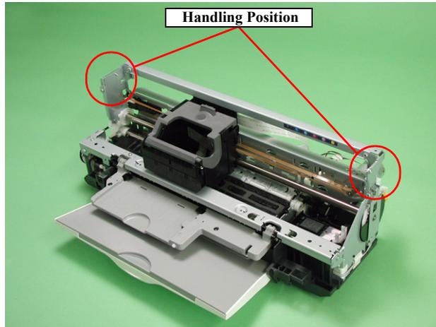
Figure 2-33. Handling Position of Printer Mechanism
