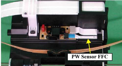
2. Check if the PW Sensor is not damaged.<br>3. Check if the PW Sensor FFC is not broken. | 1. Connect the PW Sensor FFC to CN2 on the CR Encoder Sensor Board.<br><br>2. Replace the PW Sensor with a new one.<br>3. Replace the PW Sensor with a new one. |
