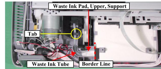
Figure 2-38. Waste Ink Tube Installation
