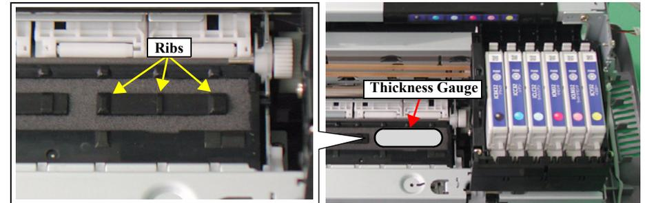
Figure 3-9. Setting the Thickness Gauge
