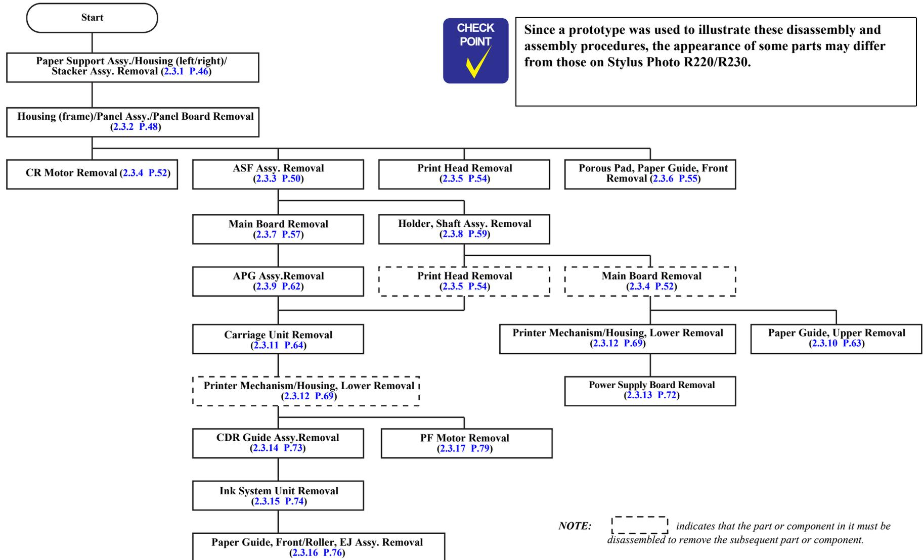
Figure 2-1. Disassembly Flowchart
