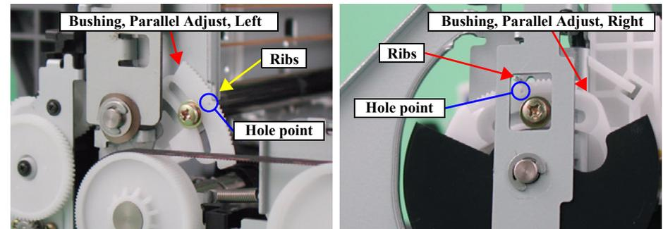
Figure 3-6. Setting the Bushing, Parallel Adjust
