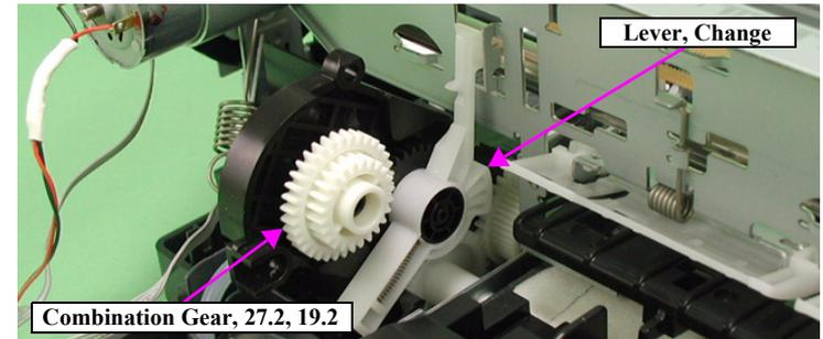
Figure 2-37. Lever, Change and Combination Gear, 27.2, 19.2
