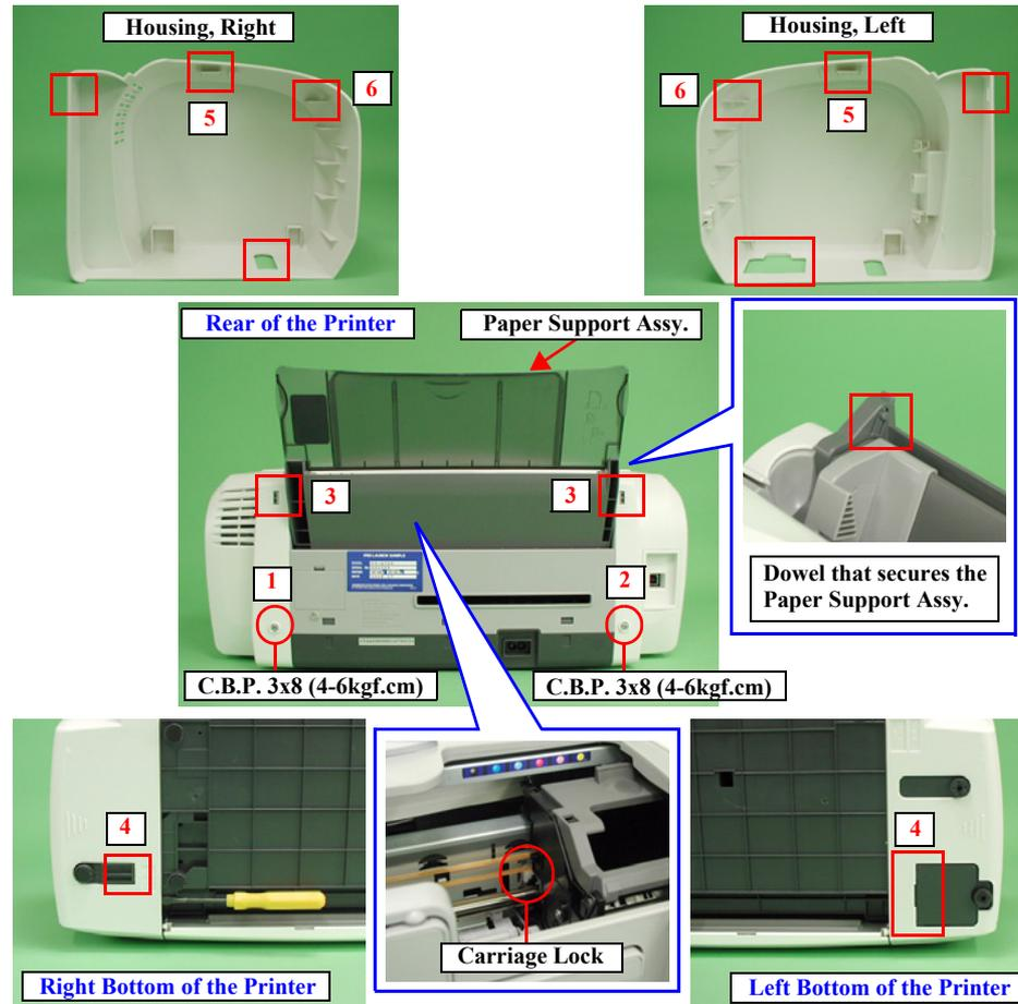
Figure 2-2. Paper Support Assy./Housing (left/right) removal
