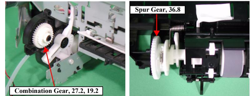
Figure 2-20. Spur Gear, 36.8 and Combination Gear, 27.2, 19.2
