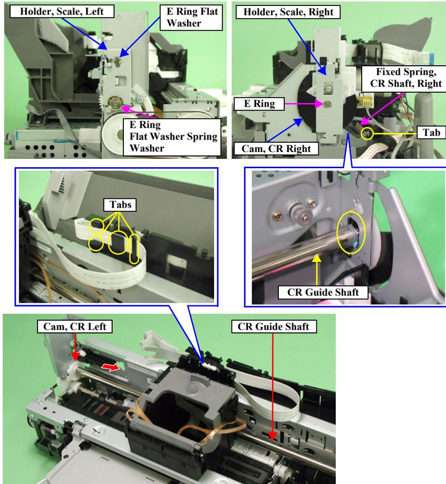
Figure 2-26. Carriage Unit Removal (2)
