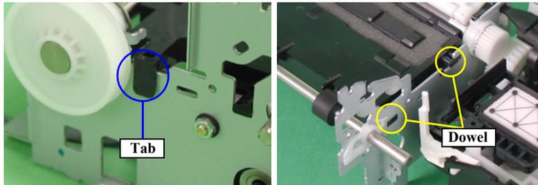
Figure 2-47. Paper Guide, Front Installation
