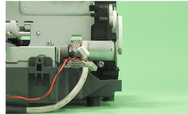
Figure 2-49. Cable connector of the PF Motor
