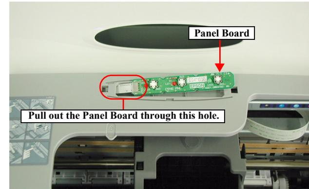
Figure 2-6. Panel Board Reinstallation
