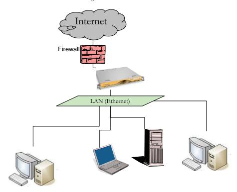
In this environment, there is no need for any agent to reside on the client machines. When any machine connects to the LAN, even temporarily, the organization's Internet usage policy is automatically enforced.
