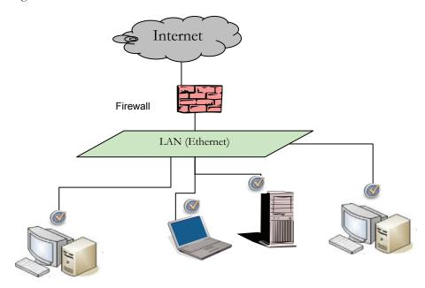
A client-side filtering solution implies that an agent is installed on each machine within the LAN. The agent (depicted in the above diagram as the ContentProtect checkmark) monitors individual machines' access to the Internet. The agent monitors all activity that originates from the machine as well as all incoming data from the Internet. If a user attempts to access something that violates the corporate Internet usage policy, the content is blocked before it displays on the computer.
