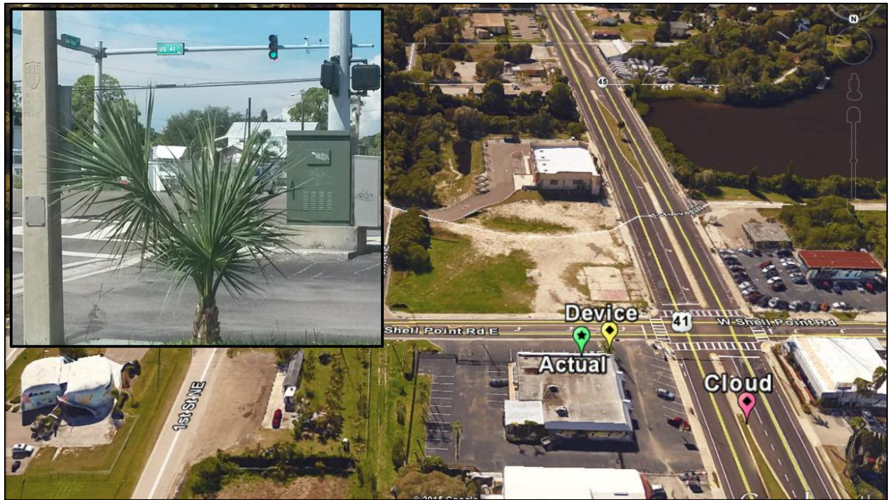
Figure 30 - Actual, Device, & Cloud locations with all sensors active (errors from 5 to 45 meters)
