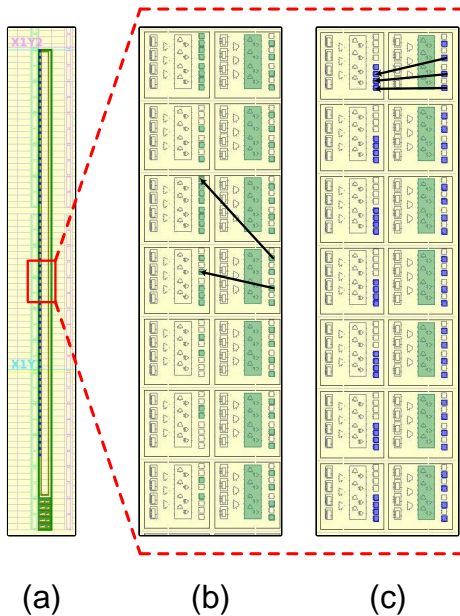
Fig. 6: (a) FPGA device view of the TDC-based sensor. The zoomed version of the section of sensor enclosed in the red box are shown in Fig. 6 (b) and (c). (b) The Vivado tool automatically places the FPGA primitives corresponding to the sensor, leading to unequal net delay between the different latch-flip-flop pairs. (c) The attacker judiciously places the FPGA primitives such that there is an approximately equal net delay between the different latch-flip-flop pairs.
