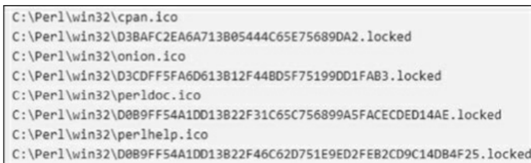
Figure 3-6: File paths in the Files tab of the Summary pane, suggesting that our sample is ransomware
