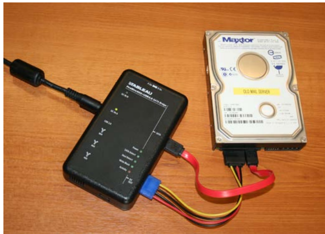
Figure 2.1 Tableau SATA/IDE Bridge Hardware write blocking device (Adapted from: URL Wikipedia, https://en.wikipedia.org/wiki/Forensic_disk_controller ).
