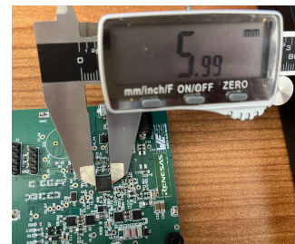
Figure 20: Microcontroller chip on the wireless charger
