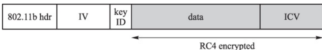
Figure 6.4 802.11b MAC sublayer frame layout
